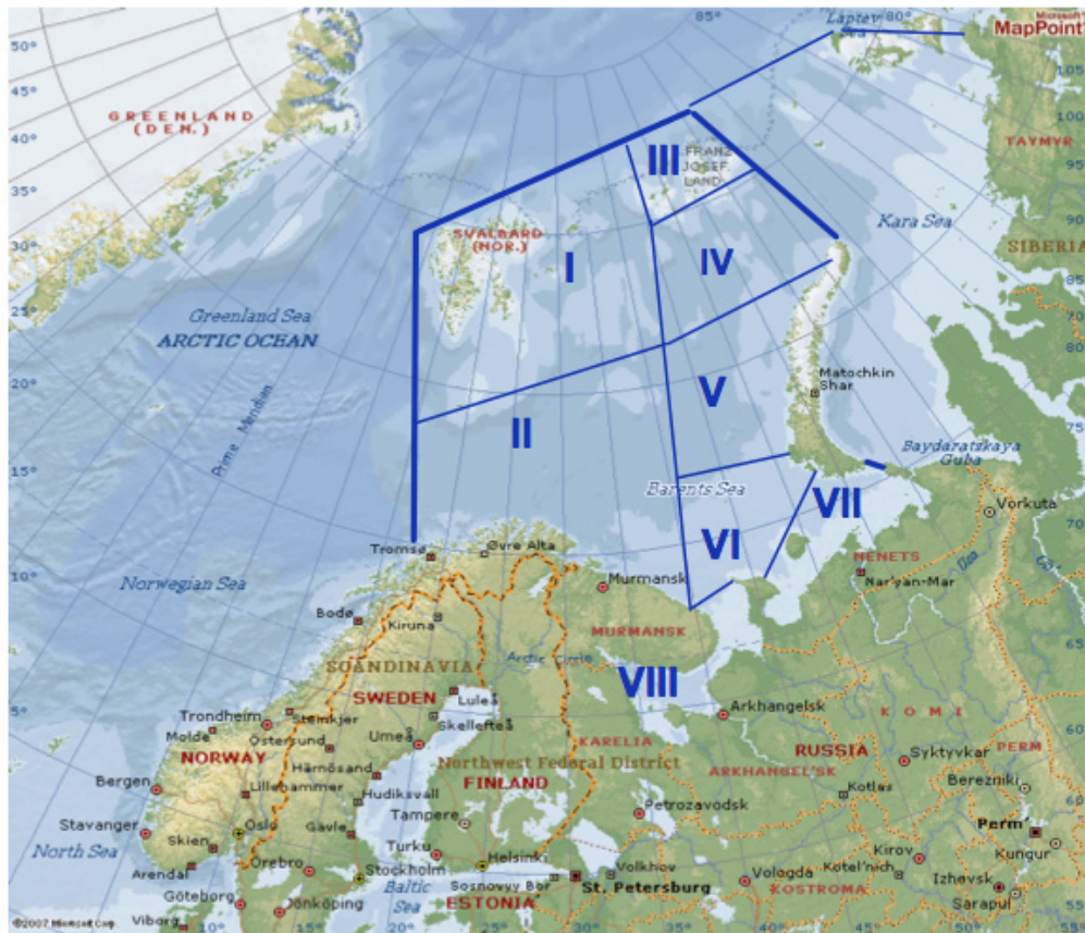
Figure A-1. Borders and sub-areas of the Barents Sea. The bold lines show the borders. The sub-areas are (modified from AARI): I) Spitsbergen; II) Norwegian; III) Franz Josef Land; IV) Northeast Barents Sea; V) Novozemelsky; VI) Kola; VII) Pechora; VIII) White Sea. Sub-area II is generally ice-free. Sub-areas I, III, IV, VII and VIII usually have ice every winter. Sub-areas V and VI are in-between. (Eide, 2008)
