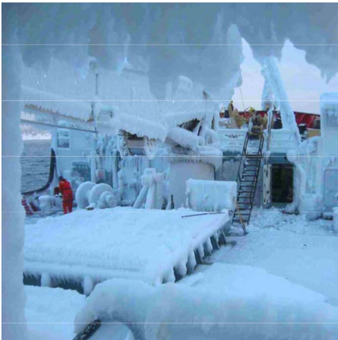
Figure B-3. Icing on deck, reels and equipment. (thenauticalsite.com, n.d.)
