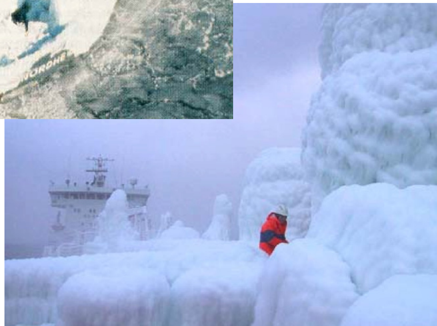
Figure B-6. Removing icing on-board deck vessel (Bergen Tanker Brokers, n.d.)
