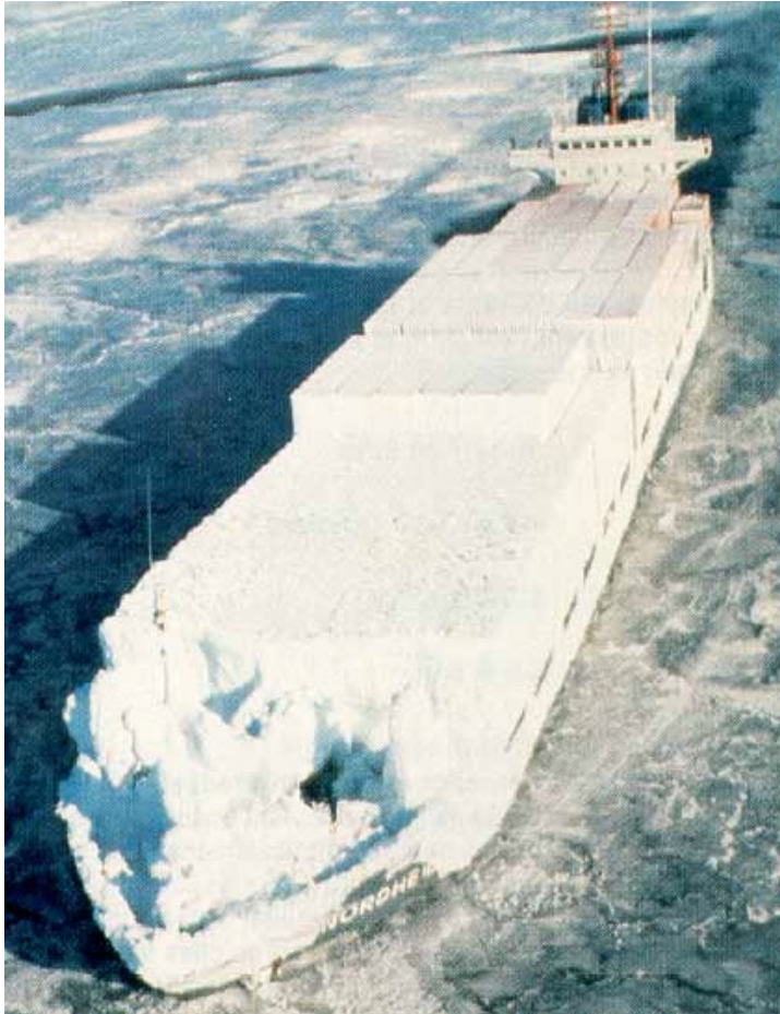
Figure B-5. Icing of winterized Arctic vessel. (Meteorological Service of Canada, 2002)
