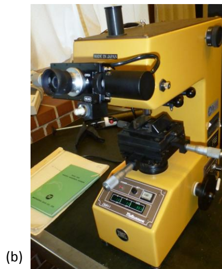
Figure 39. Hardness testers: (a) Wolpert Wilson universal hardness tester, model 930, used for Rockwell hardness testing. (b) Matsuzawa DMH-1 micro hardness tester used for Vickers hardness testing.
