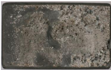
Figure 66. Approximately all pitting corrosion has occurred on one of the (2,5x1,5) cm face on the HVOF test specimens.
