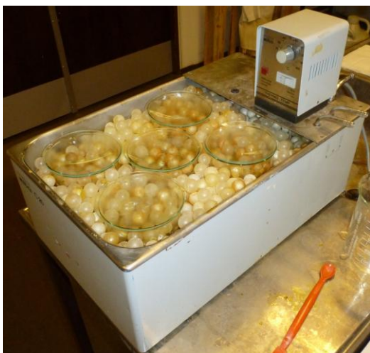
Figure 55. Test setup of the corrosion G48 test showing the temperature controlled water bath with submerged glassware. One glass container for each treated duplex; untreated duplex, Expanite, Kolsterising, HVOF and Sursulf. The water bath and the \text{FeCl}_3 solution are covered by balls for insulation and evaporation purposes.
