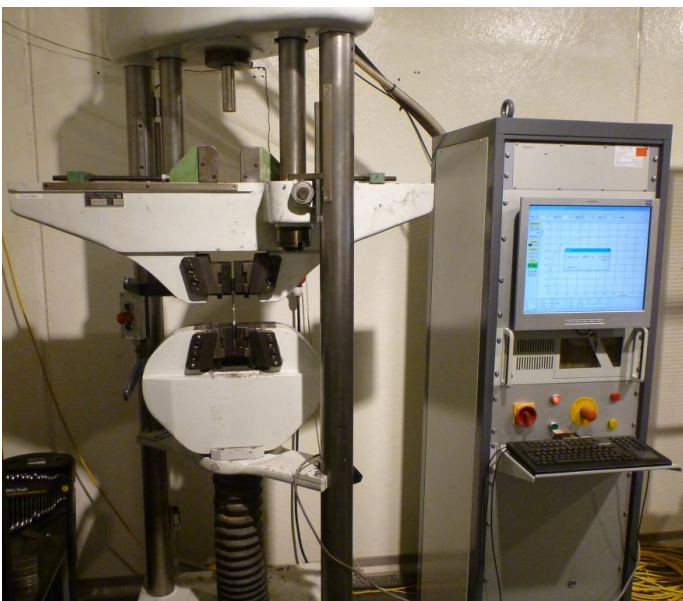
Figure 36. The tensile testing machine, Schütz+Licht Prüftechnik GmbH – Wolpert U60, to be used on the tensile test at Quality lab. facility in Forsand.
