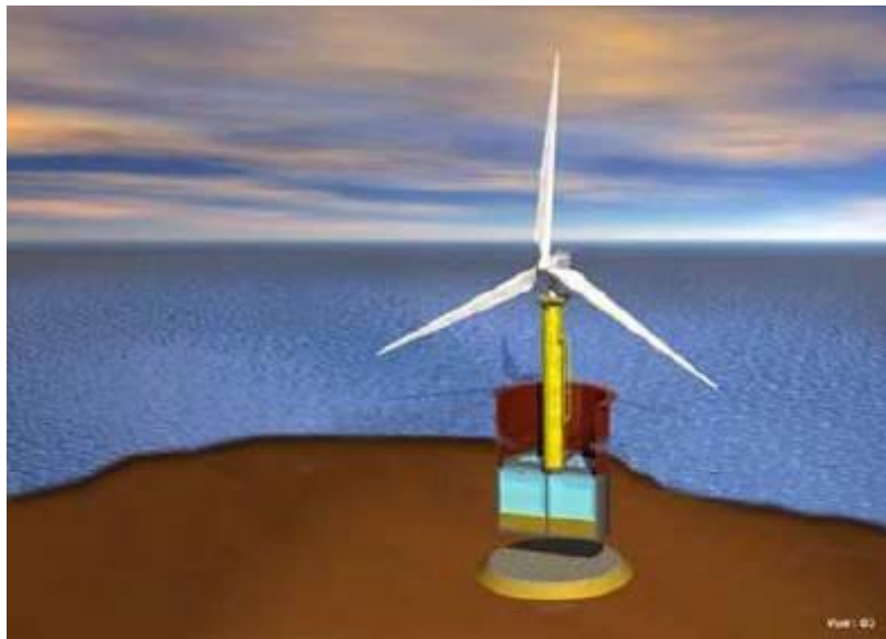
Image 3: Fully assembled wind turbine settled on a foundation offshore with pontoon connected, with a telescopic joint [15].
