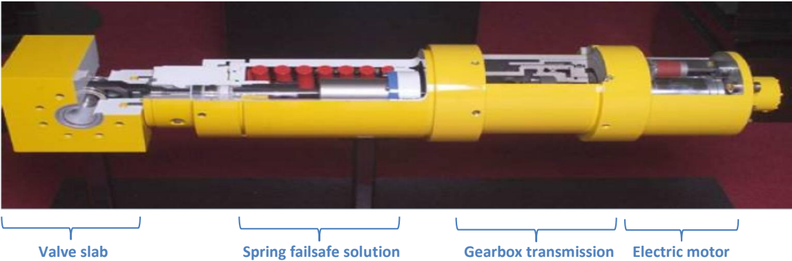
Picture 4: Cameron all-electric gate valve (MacKenzie, Rory; Total E&P, 2011)
