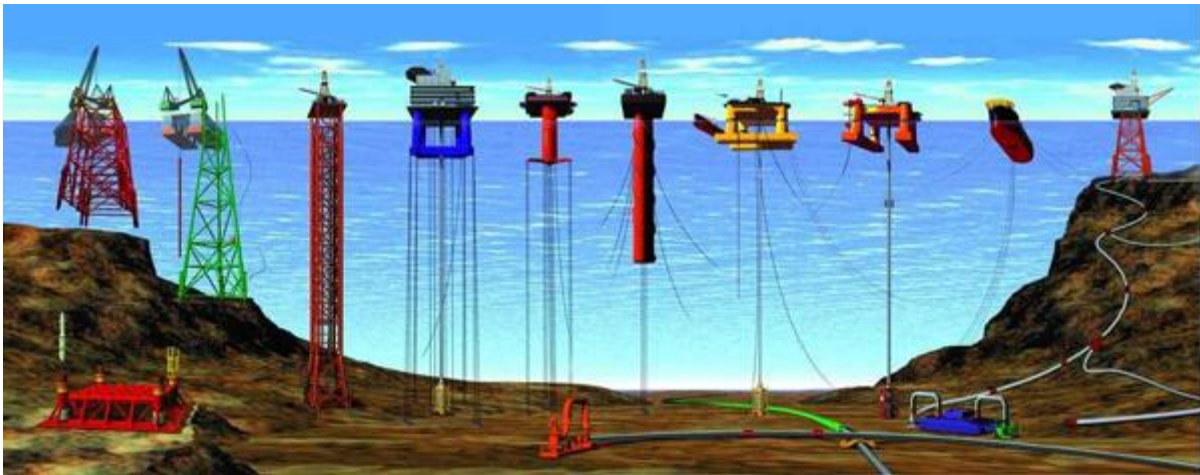
Figure 1: Surface facility designs used in oil & gas production systems (National Oceanographic and Atmospheric Administration, 2012)
