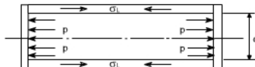
Figure 2-8: Pressure induced by End Cap Effect (Karunakaran, 2012)
