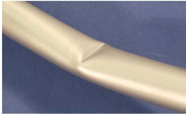
Figure 1-4: Example for Ovalisation Failure Mode (Kyriakides and Corona, 2007)
