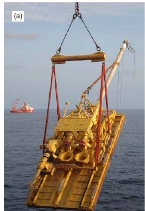
Figure 1-21: PLET with Sliding Foundation (Carneiro and castelo, 2010)
