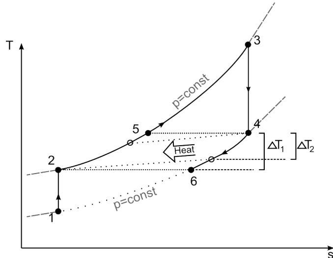
Illustration 10: Ideal and real recuperator in a Brayton cycle in the  $T - s$  dimensions
