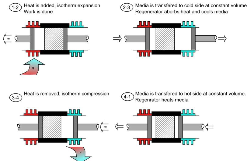
Illustration 22: Simplified workings of a Stirling engine
