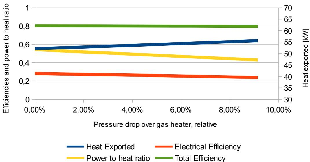
Chart 3: Power to heat ratio, total- and electrical efficiency and heat exported, as function of pressure losses over the gas heater. The heat exported is again plotted against the right axis.
