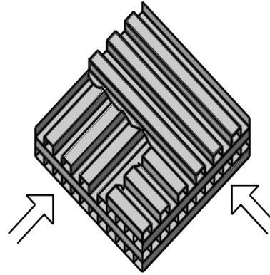
Illustration 5: Crossflow plate-fin design heat exchanger
