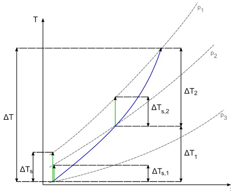
Illustration 26: An compression process in the T-s dimensions
