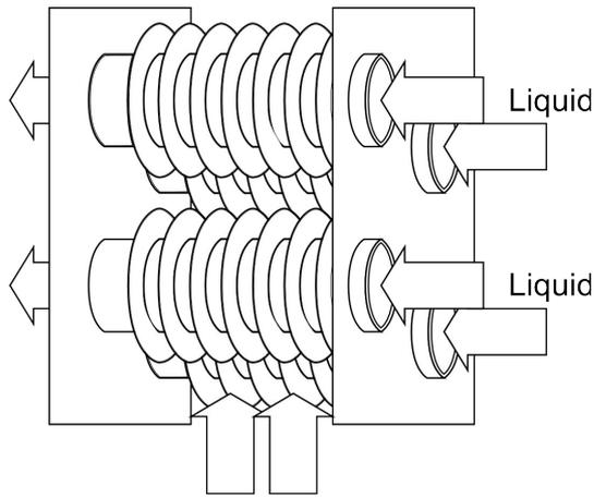
Illustration 4: Crossflow finned tube design heat exchanger
