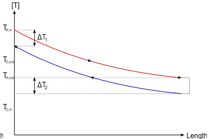
Illustration 7: Temperature as a function of length in a counterflow heat exchanger
