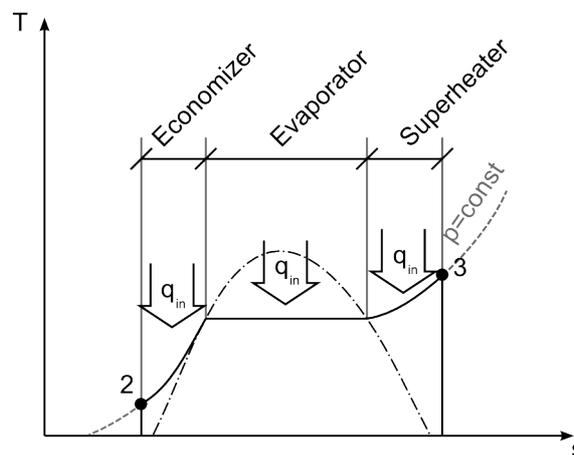
*Illustration 17: The boiler is divided into the economizer, evaporator and superheater, by the phase the fluid is in*
