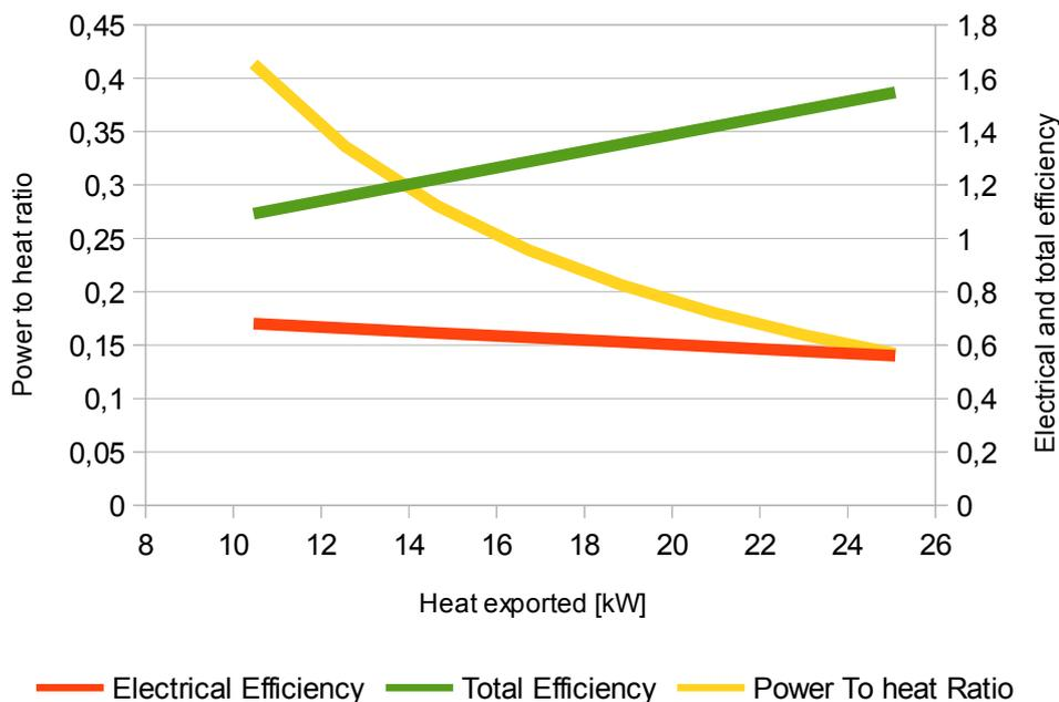
Chart 10: Electrical and total efficiency, and power to heat ratio as function of exported heat in layout 2
