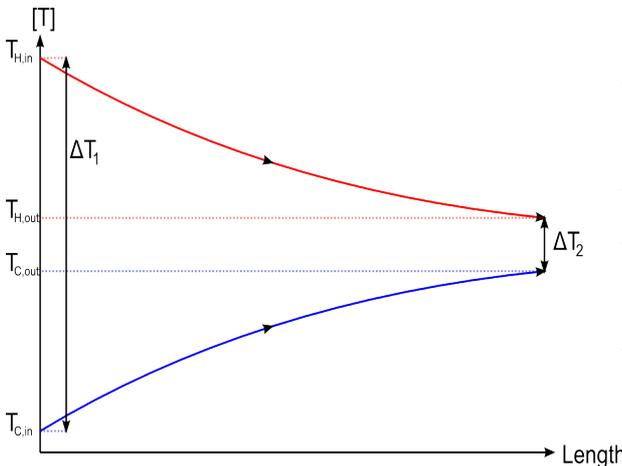
Illustration 6: Temperature as a function of length in a parallel flow heat exchanger
