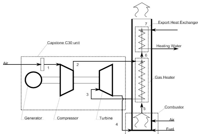
*Illustration 30: Layout of CHP plant with air feedback into the combustor, and gas heater placed before export heat exchanger in the flue gases.*
