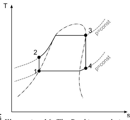
*Illustration 16: The Rankine cycle in an  $T-s$  diagram with an organic liquid with a positive vapor curve as the working fluid*
