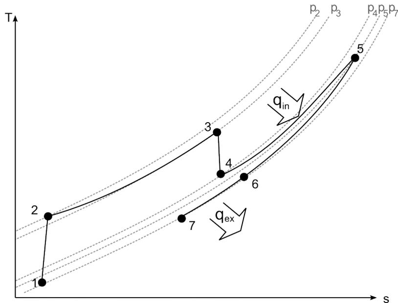
Illustration 31: The Brayton cycle with air feedback, gas heater and export heat exchanger
