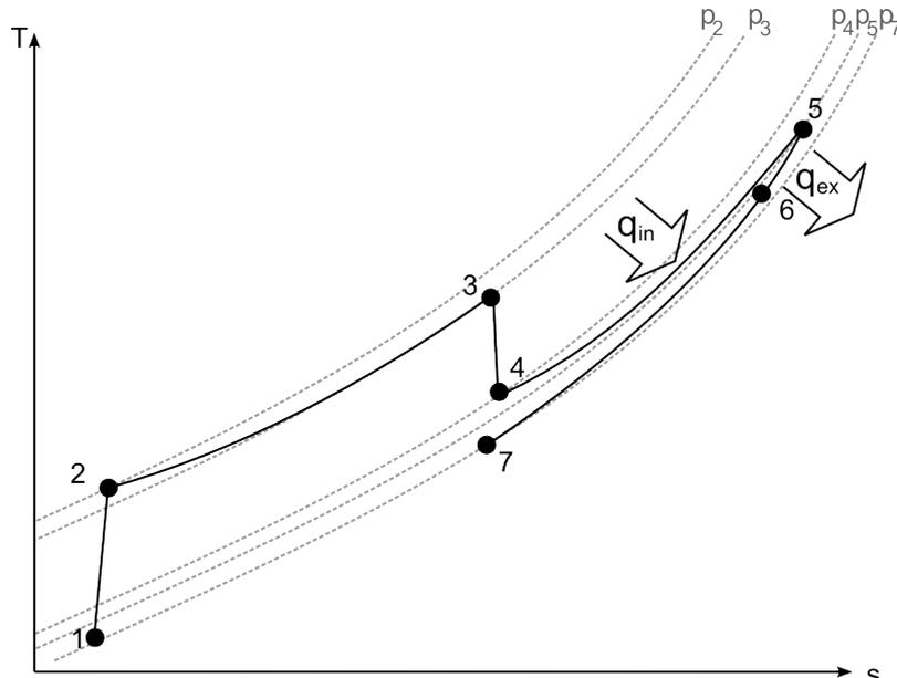
*Illustration 33: T-s diagram of the Brayton cycle for layout 2*
