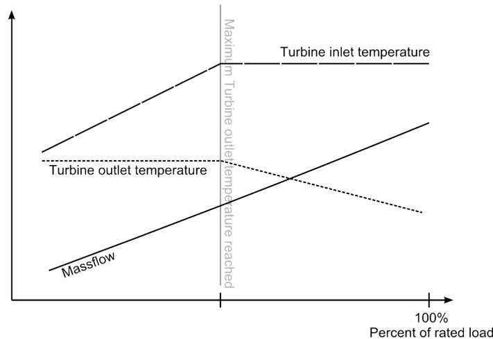
*Illustration 28: Mass flow and turbine inlet and outlet temperature as function of reduction in load*
