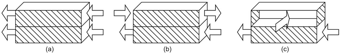
*Illustration 3: The three main flow designs of heat exchangers. (a) Parallel flow, (b) counterflow and (c) crossflow*
