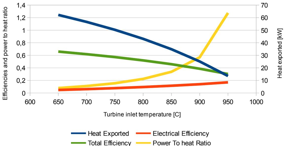
Chart 9: Power to heat ratio, total- and electrical efficiency and heat exported, as function of the turbine inlet temperature for layout 2. Heat exported is plotted against the left y-axis.
