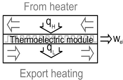
*Illustration 24: Thermoelectric cells placed between the hot and cold side of an heat exchanger to create electrical power*
