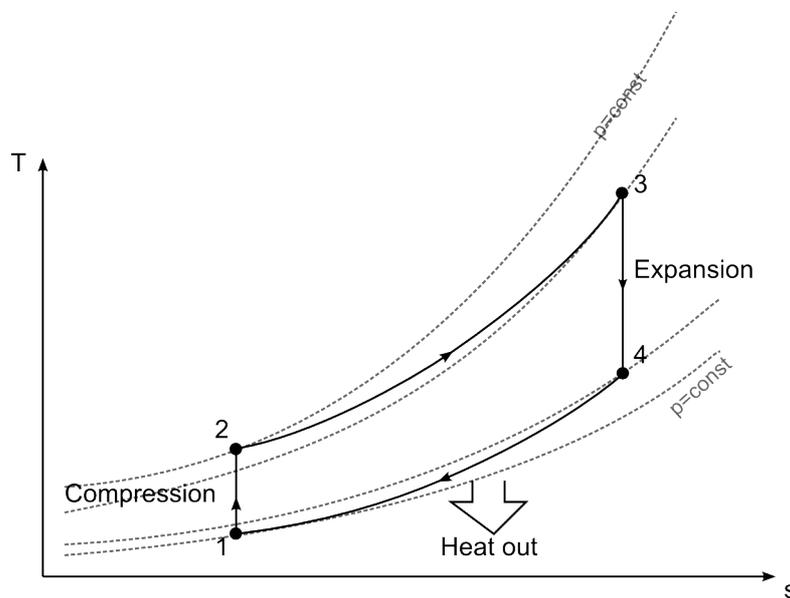
Illustration 13: Pressure drop over gas heater and recuperator illustrated in a *T - s* diagram
