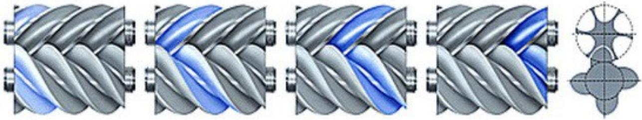
*Illustration 19: Screw compressor. Image of an Atlas Copco ZT/ZR 110-900 rotary screw compressor. [ESI.info, 2013]*
