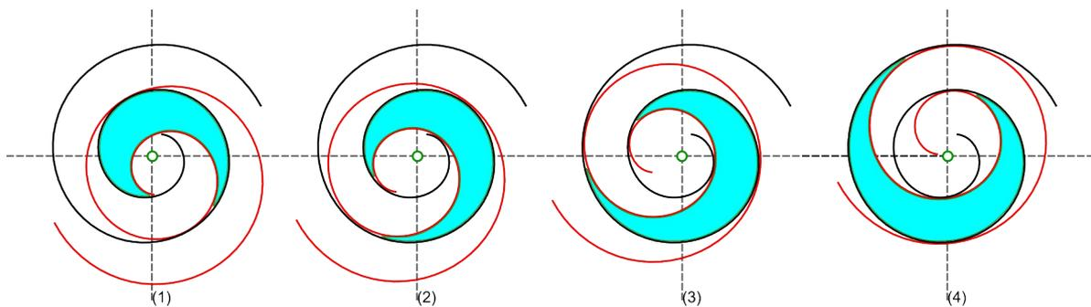
*Illustration 20: Workings of an scroll expander. As the fluid expands, the red scroll is moved around without rotating.*
