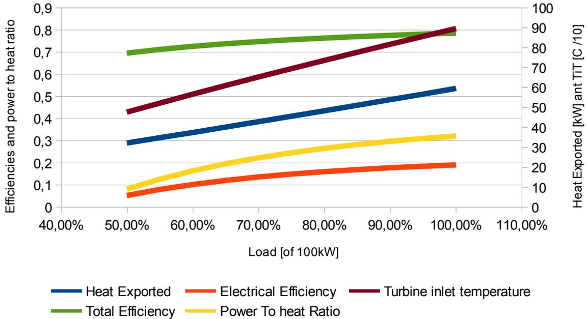
Chart 7: Part load performance with varying TiT and constant mass flow for Layout 1
