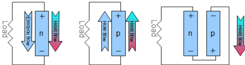
*Illustration 23: Thermoelectric blocks of the n- and p- types, and a thermocouple*
