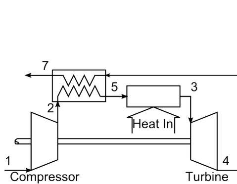
Illustration 11: System sketch for a gas turbine with recuperator
