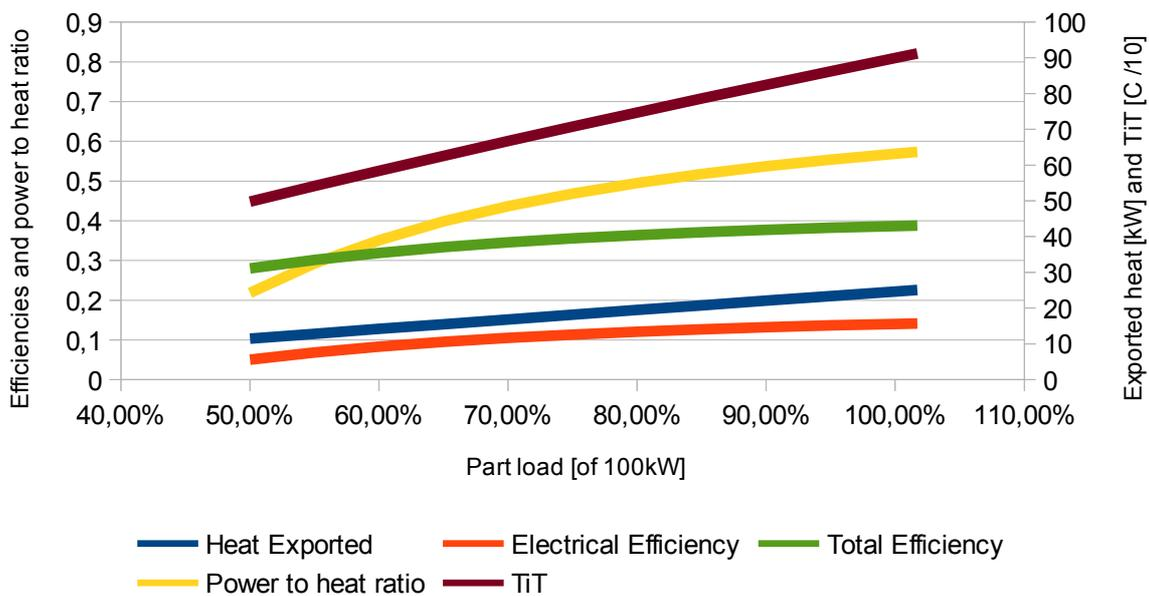
Chart 11: Part load performance with varying TiT and constant mass flow for Layout 2
