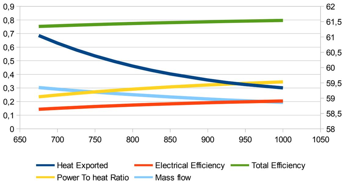
Chart 6: Power to heat ratio, mass flow, total- and electrical efficiency and heat exported, as function of the turbine inlet temperature for layout 1.
