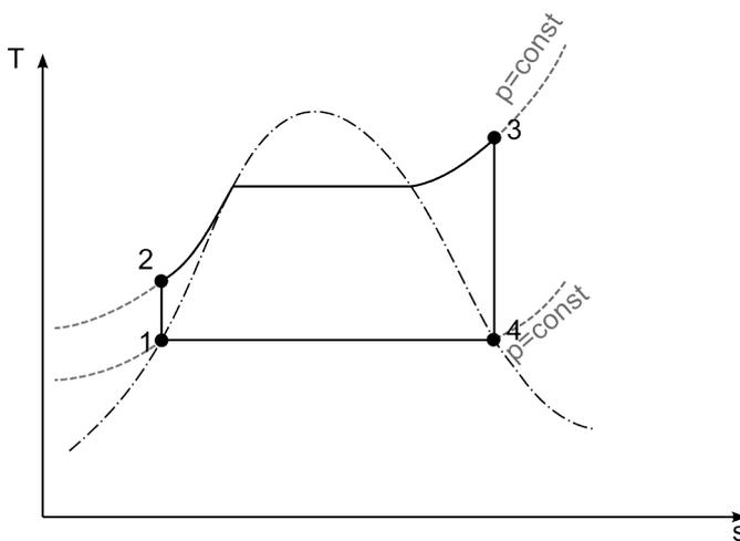
*Illustration 15: The Rankine cycle in an  $T-s$  diagram with water as the working fluid*
