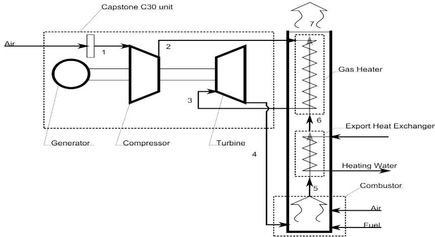
*Illustration 32: Layout of CHP plant with air feedback, and export heat exchanger placed before gas heater in the flue gases.*
