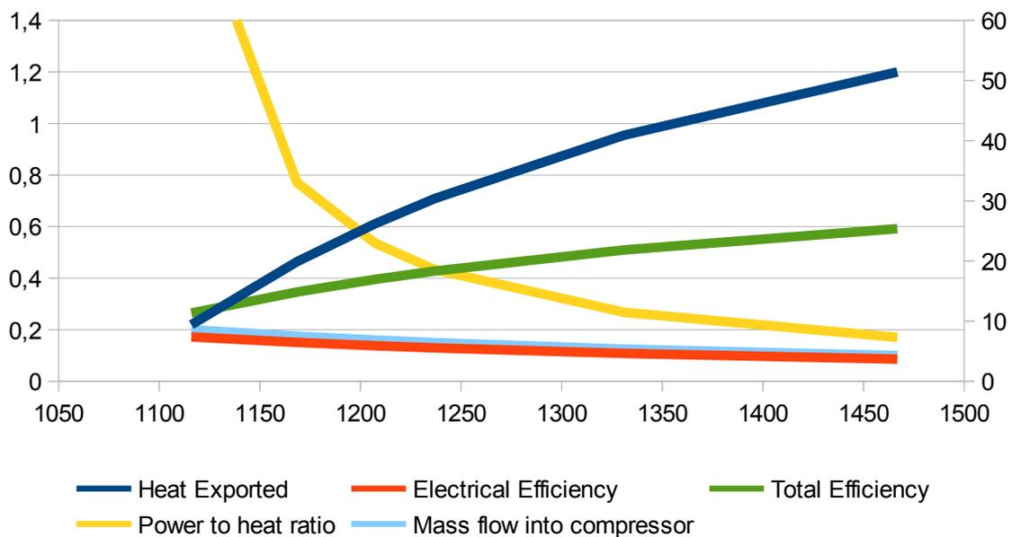
Chart 8: Efficiencies, heat exported, power to heat ratio and mass flow as function of combustion chamber outlet temperature
