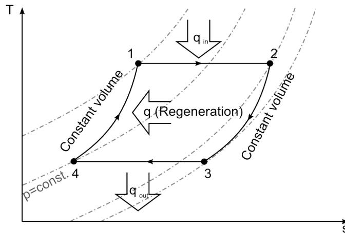
Illustration 21: The Stirling cycle in a T-s diagram
