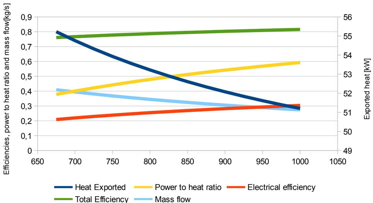
Chart 2: Power to heat ratio, mass flow, total- and electrical efficiency and heat exported, as function of the turbine inlet temperature for the base case.
