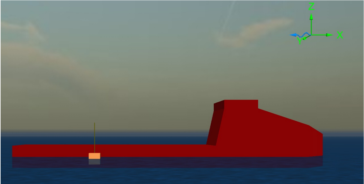
Figure 2-6 Module lift partly submerged
