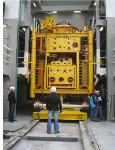
Well Control Package
