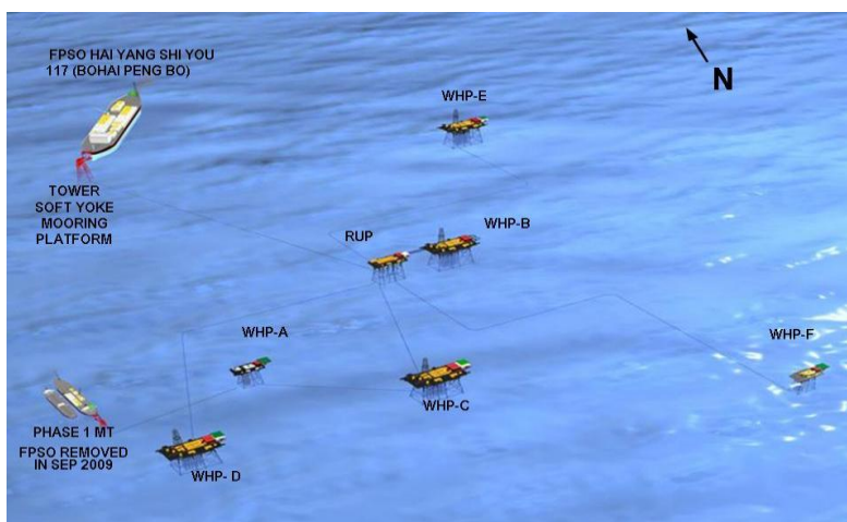
Figure 4.6 The layout of the Penglai 19-3 oilfield [made by author]
