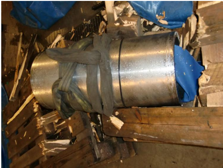
Figure 6-30: Test Casing after Test Failure of Alt. 2
