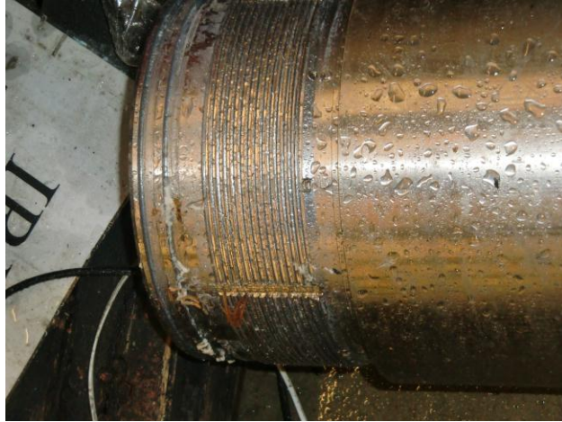
Figure 6-27: End Coupling Alt.2 after Test Failure
