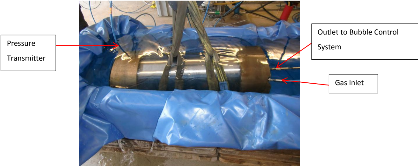
Figure 6-12: Test Assembly 1 in Water Tank at IRIS
