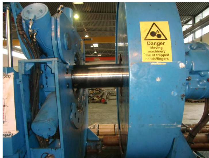
Figure 6-8: Use of Torque Machine to Assemble Test Equipment on Alt. 1
