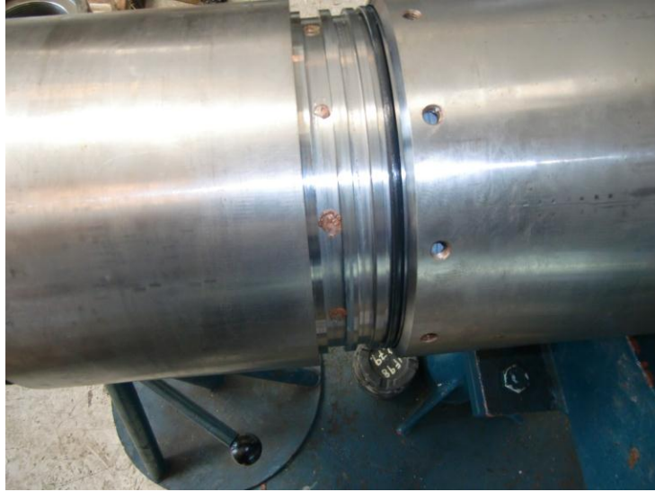
Figure 6-24: Seal Alt.1 after Pressure Test
