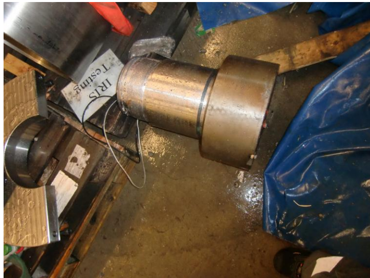
Figure 6-28: End Coupling Alt. 2 after Test Failure
