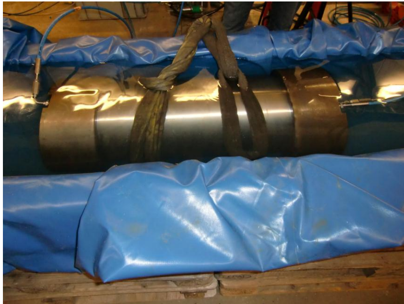
Figure 6-17: Test Assembly 2 Installed for Pressure Test
