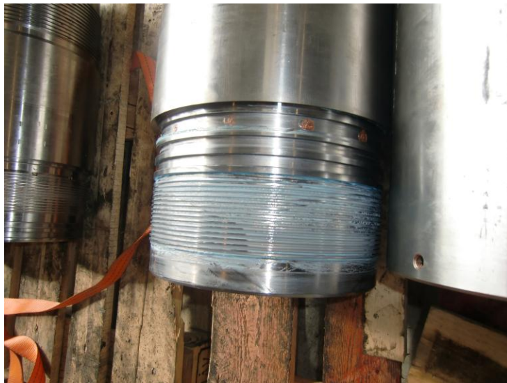
Figure 6-24: Seal Alt.1 after Pressure Test
