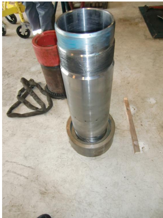
Figure 6-6: Test Cap Mounted on End Coupling of Alt. 1
