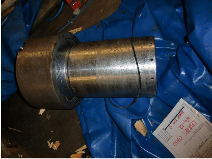
Figure 6-29: Housing Alt. 2 after Test Failure
