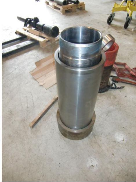
Figure 6-7: Test Casing Fitted over Test Piece of Alt. 1
