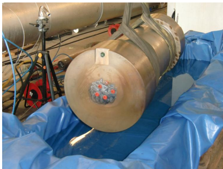
Figure 6-16: Installing Test Assembly 1 for Second Pressure Test
