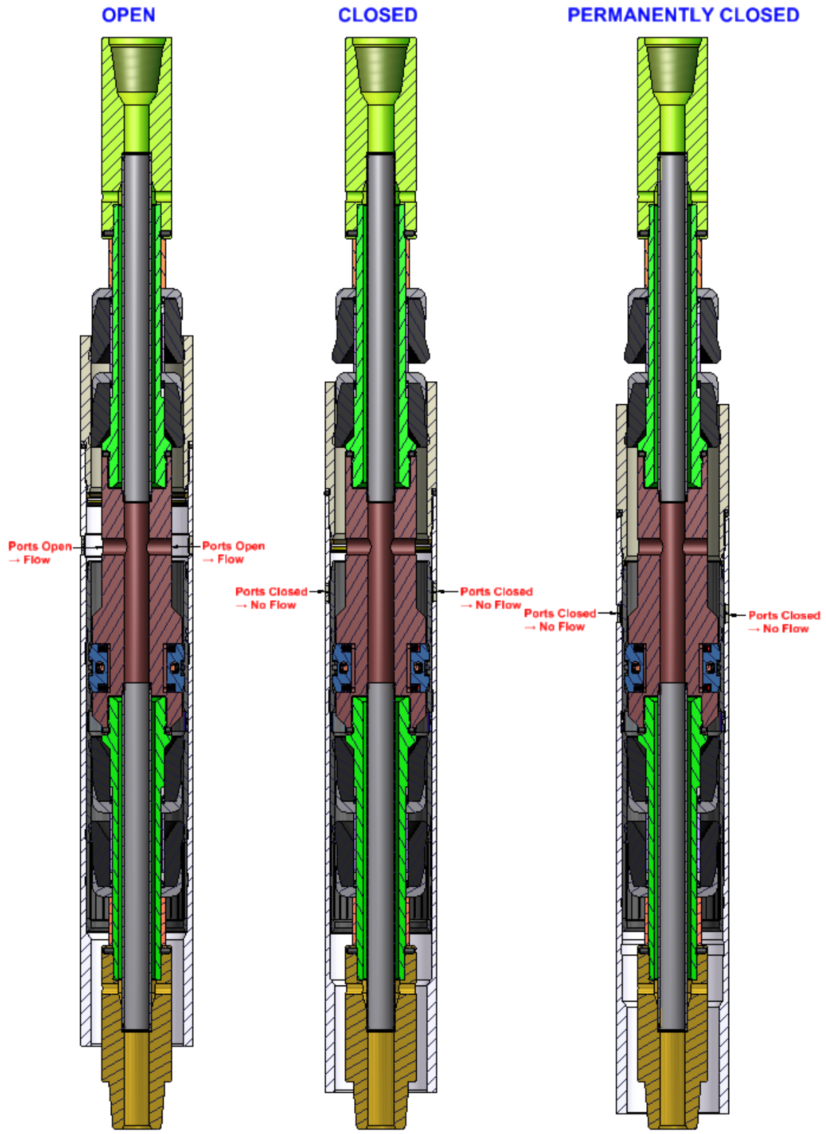
Figure 4-2: C-Flex SS 9 5/8" 53# with Cementing Tool in Open, Closed and Permanently Closed Position [1]
