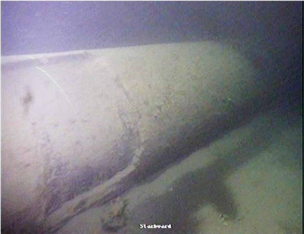
Figure 2-53 Typical damage to filler joint (Polyurethane filler), where corrosion coating is exposed at field joint.
