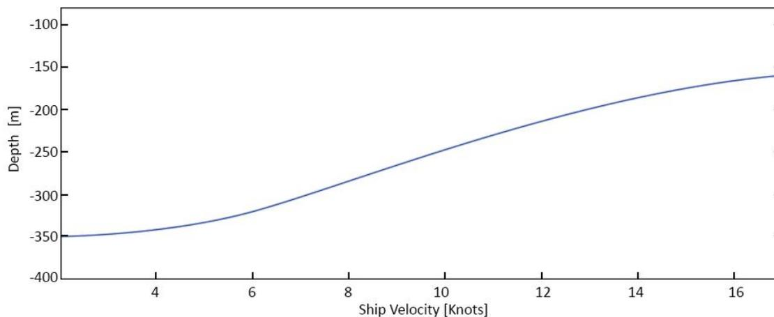
Figure 3-14 Maximum 13500 kg Anchor Tow Depth for Versus Ship Velocity (Source: Vervik, 2011)
