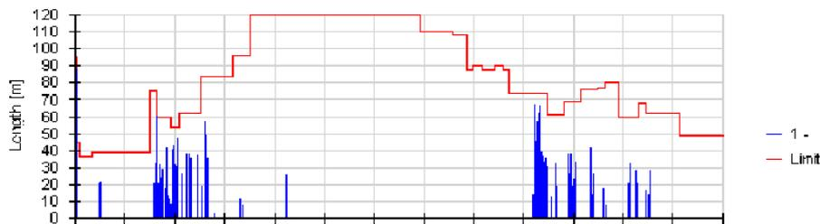
Figure 2-68 Free span lengths within a certain leg of the GNG pipeline. Source: Annual GNG pipeline inspection 2012
