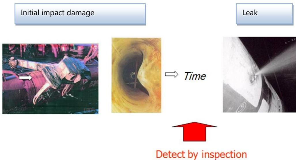
Figure 2-65 Pipeline leak developing over time (Gassco, n.d.b)
