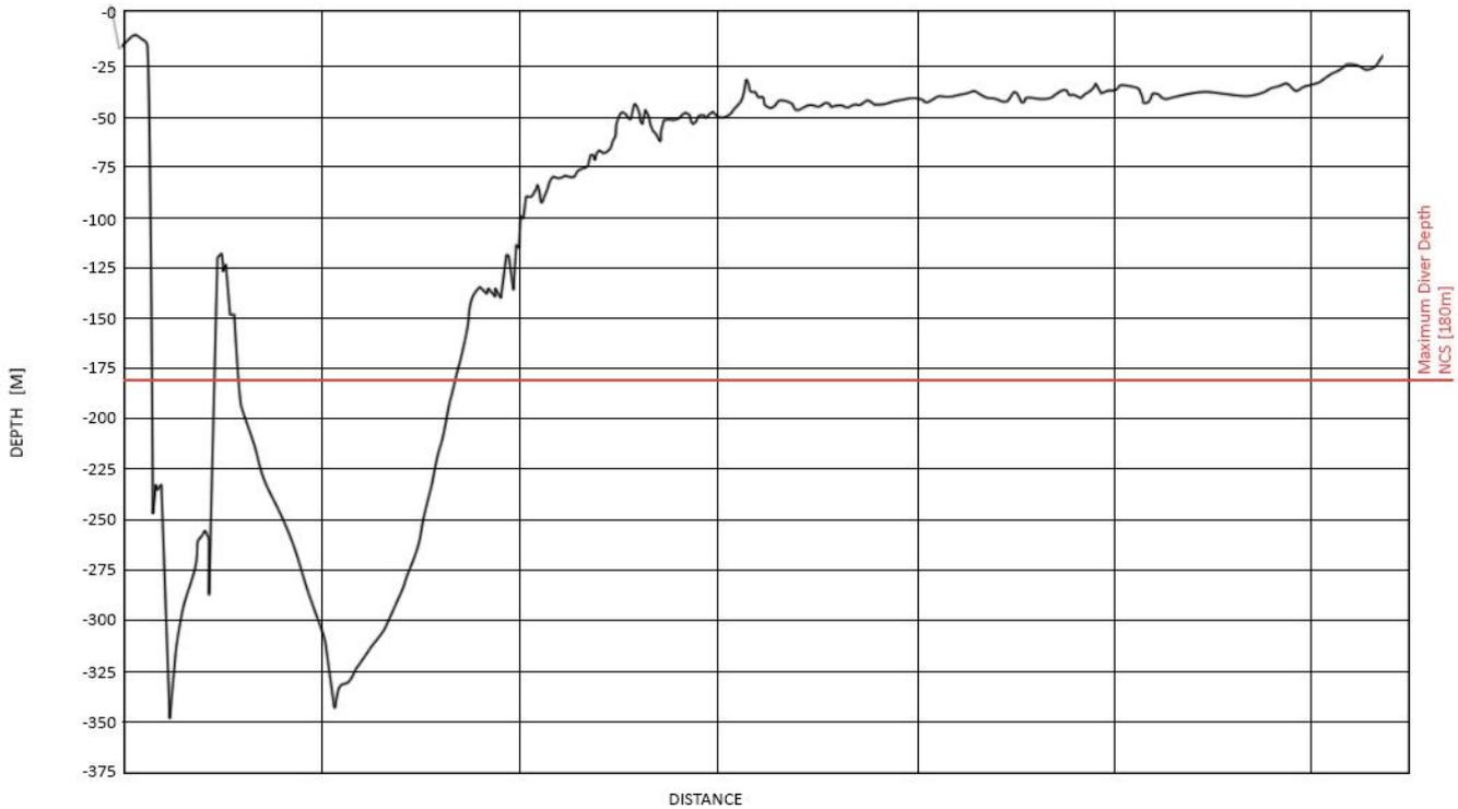
Figure 2-66 GNG Pipeline Profile with diver depth limitation, Source: GNG pipeline DFI
