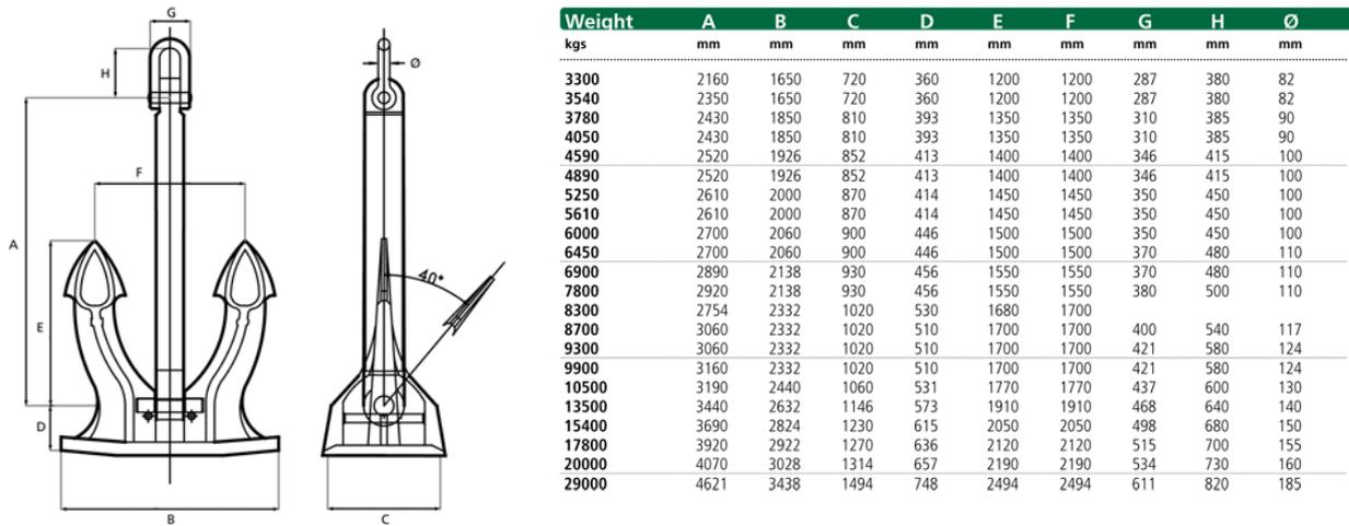
Figure 3-12 Stock Spek anchor specifications (Sotra, 2013)
