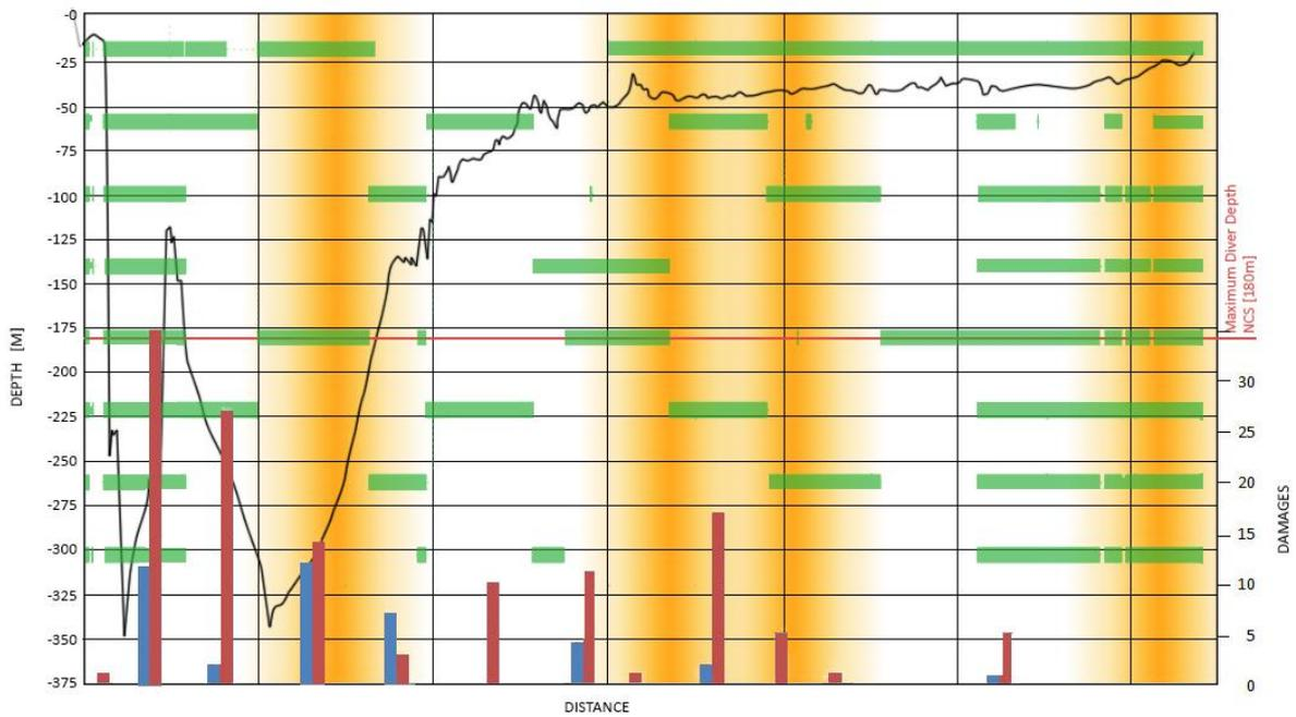
Figure 4-10 GNG pipeline profile plotted against diver depth, annual inspection coverage intervals, ship traffic and pipeline impact quantities and type.
