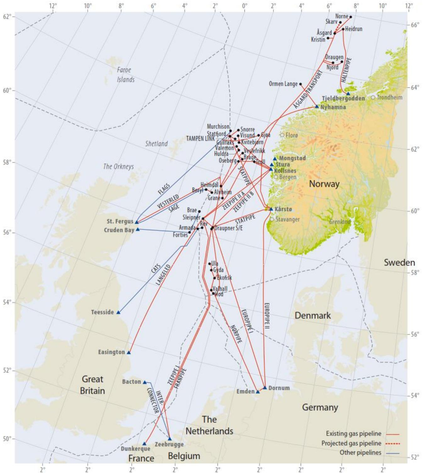
Figure 1-1 Norwegian natural gas pipeline infrastructure (NPD, 2012)
