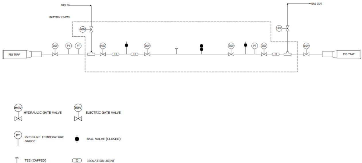
Figure 2-50 Battery limits GNG Pipeline
