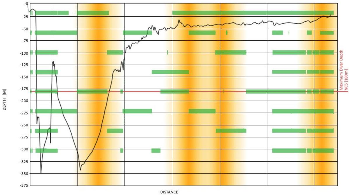
Figure 4-11 GNG pipeline profile plotted against diver depth, annual inspection coverage intervals and ship traffic
