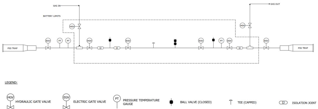
Figure 1-8 Physical Battery limits of simplified GNG pipeline Schematic. Data Source: DFI GNG pipeline
