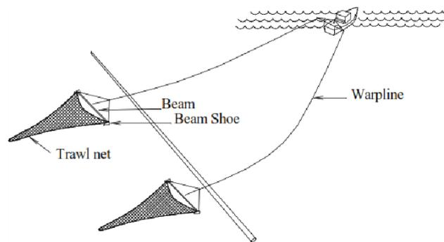
Figure 2-54 Typical beam trawl gear crossing a pipeline (DNV, 2010b)
