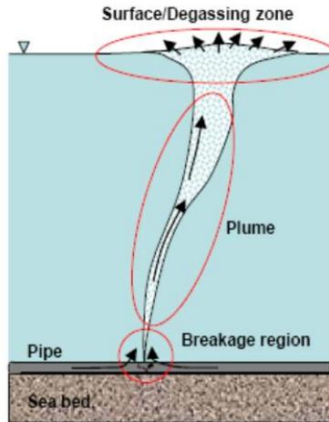
Figure 3-17 Illustration of gas leak from a ruptured subsea pipeline (Gassco, 2007)
