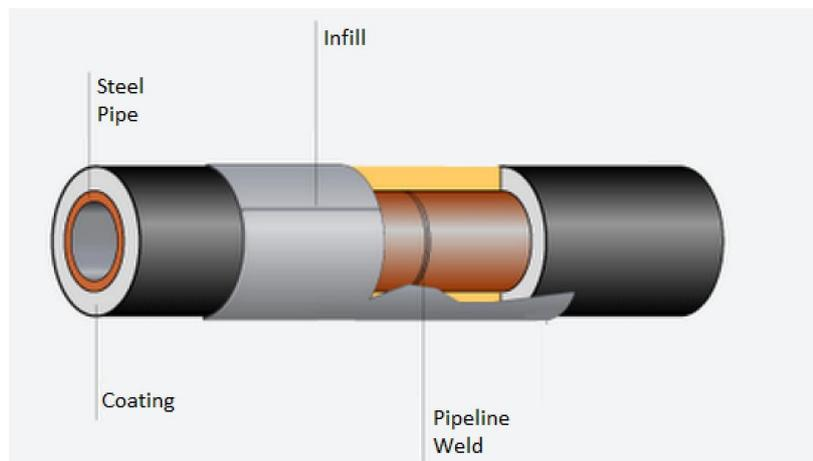
Figure 2-52 Field Joint. Source: (ASRO, 2009)
