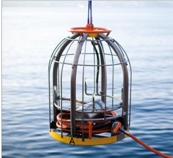
Figure 2.7 Acoustic leak detection from Naxys, left: ALD module ( naxys.no ), right: hot-spot acoustic sensor ( naxys.no )
