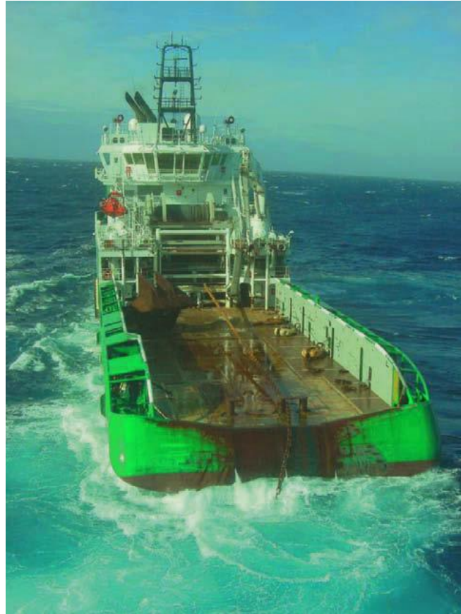
Figure 5.4 The Bourbon Dolphin with chain located between tow pins (Photo: Sean Dickson)
