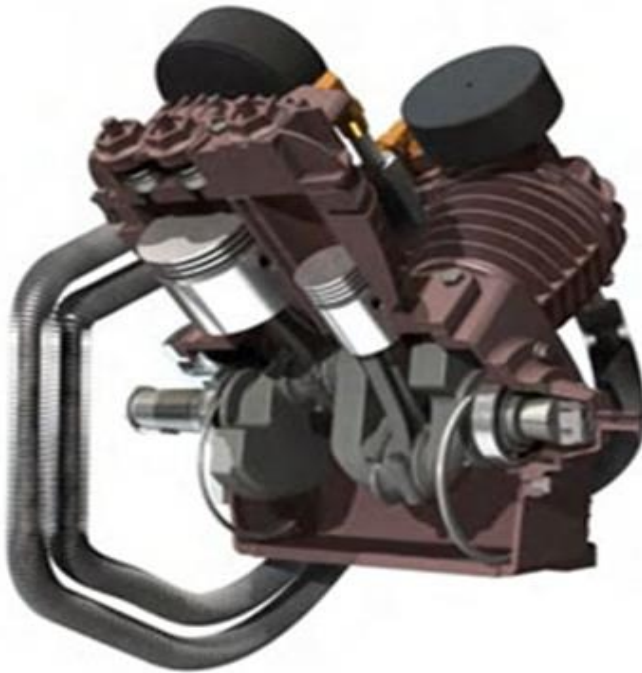
Figure 4.7 – Concept of a 4 piston compressor with V-block [8]
