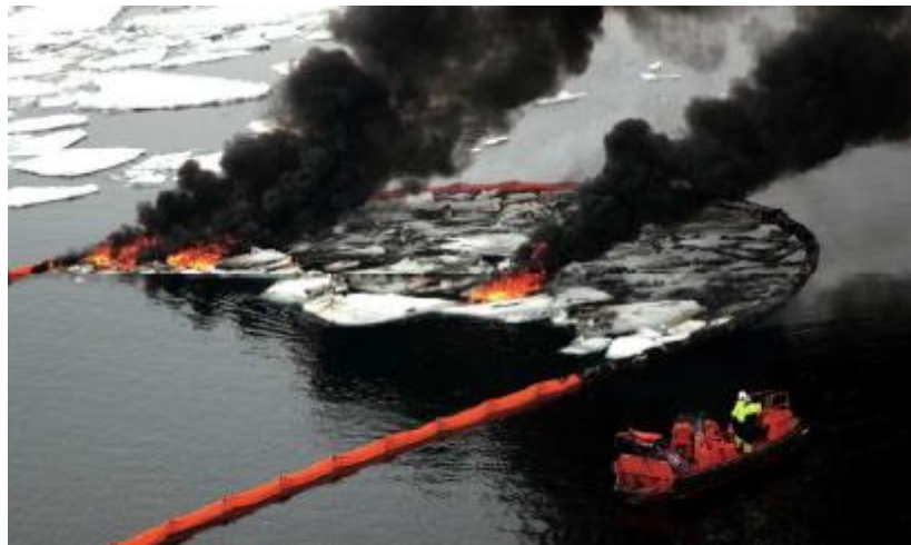
Figure 4.8 Burning oil mixed with ice cakes and pieces collected within a fire resistant boom
