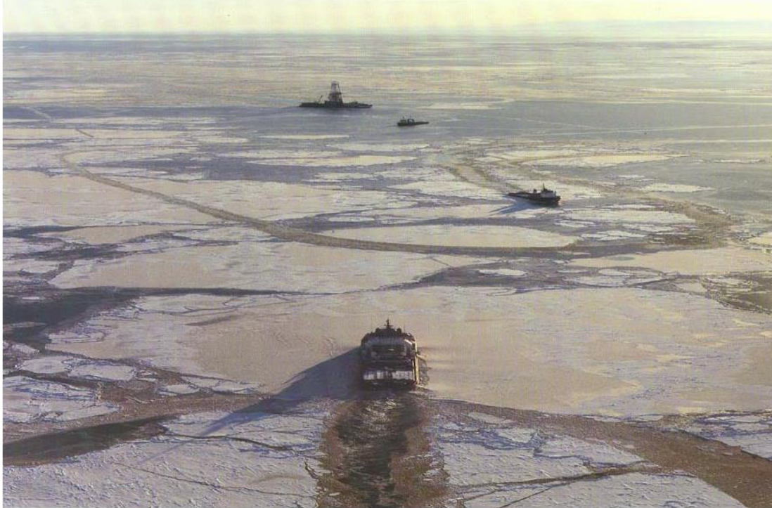
Figure 3.5 Ice management for a drill ship in pack ice Courtesy to Dunderdale, P. and Wright, B. (2005)
