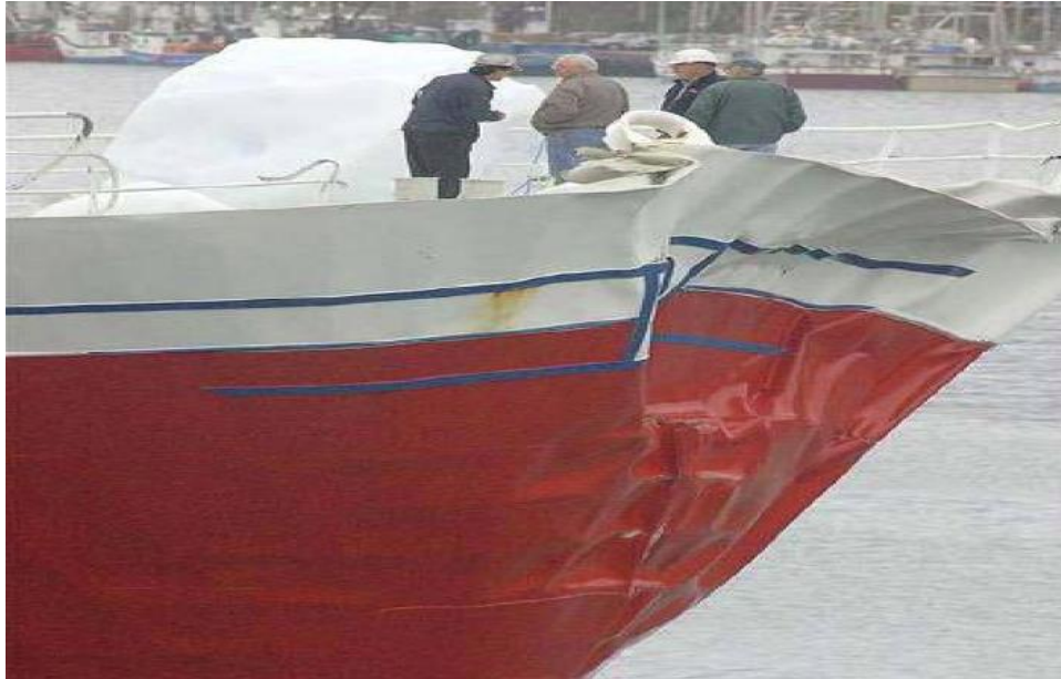
Figure 2.9 A view of ice related damage to a vessel Courtesy to Dunderdale, P. and Wright, B. (2005)
