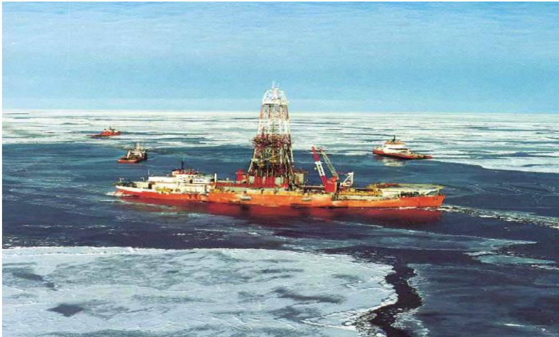
Figure 3.7 Ice management for drill ship in the Beaufort Sea Courtesy of Noble Denton Canada Ltd. & B. Wright & Associates Ltd (2005)
