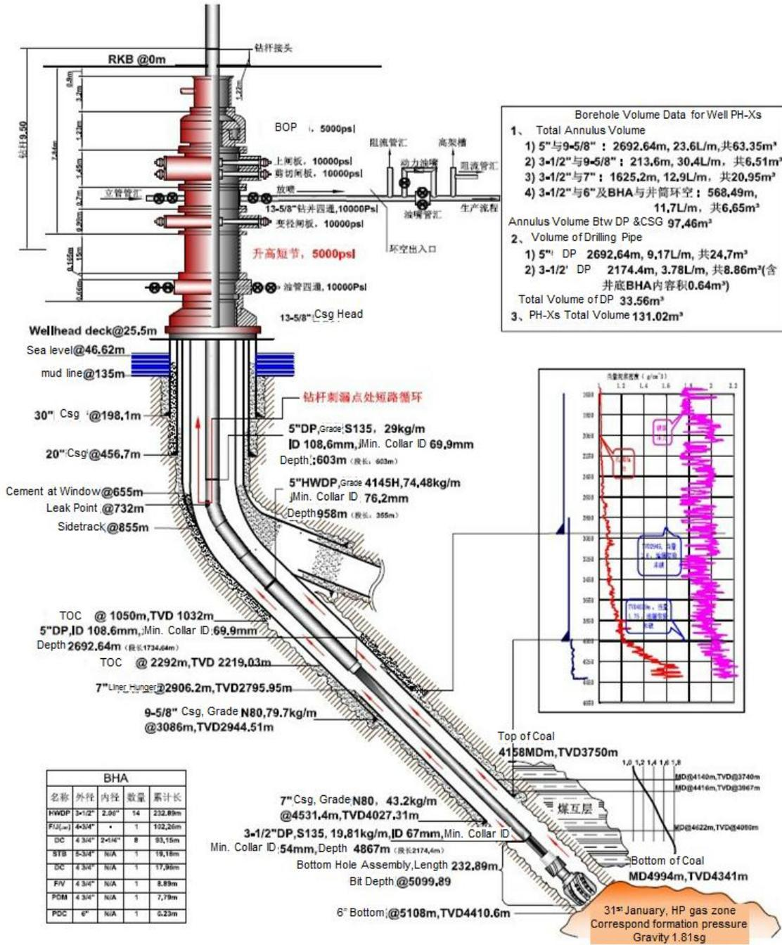
Figure 37 Well Schematic of Well PH-Xs
