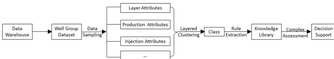
Figure 35 Data Mining Model for Oilfield Well Group Production Decision-making System
