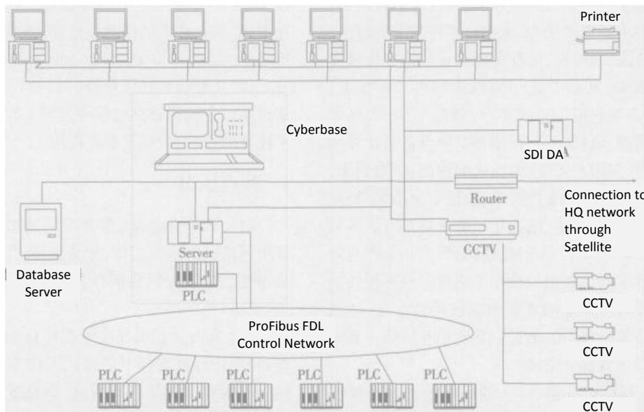
**Figure 21 Schematic of Well-site Distributed Database Management System(Zhang and Guo, 2005)**
