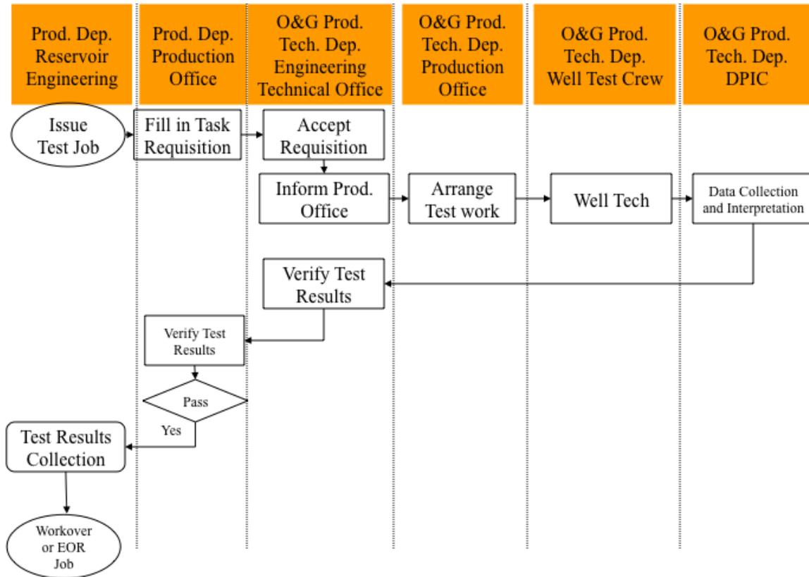
Figure 29 the Main Work Process of Well Test Job
