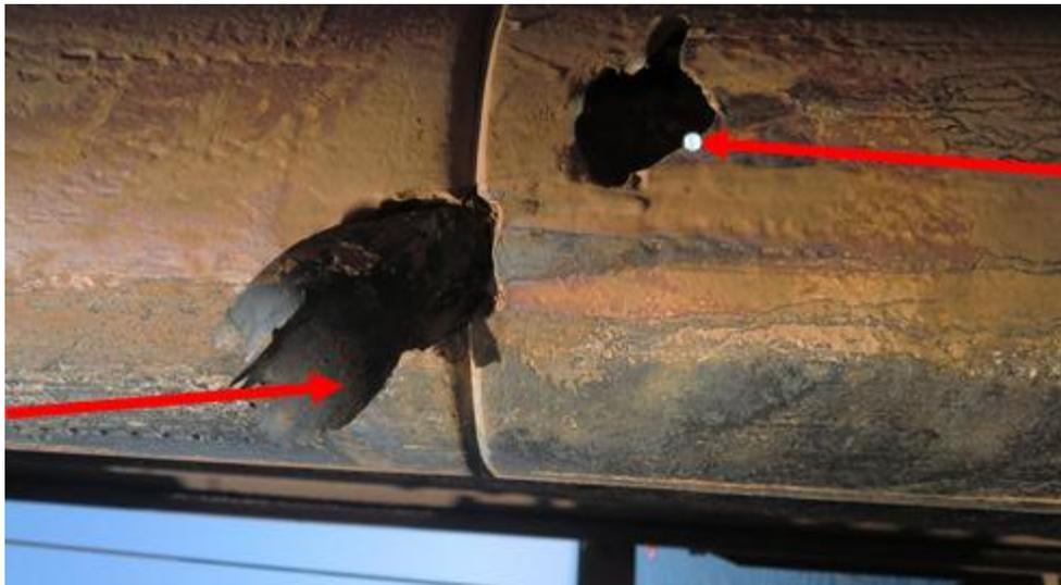
Figure 41 Photo of DP String Damage in Well PH-Xs
