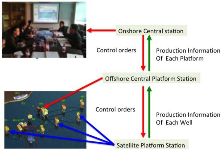
Figure 25 the Schematic of the Oilfield Microwave Communication
