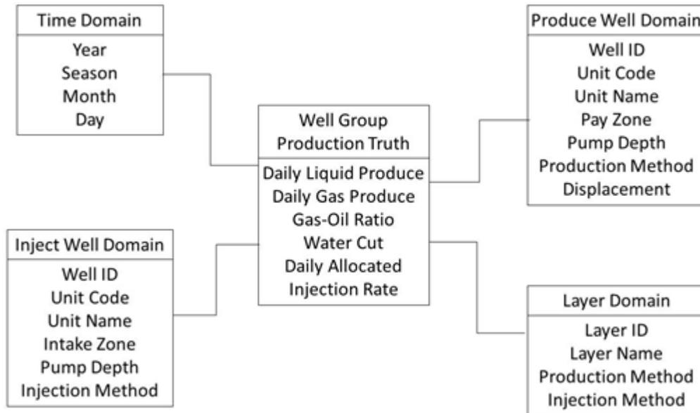
Figure 34 Multiple Domain Data Model of Well Group Production
