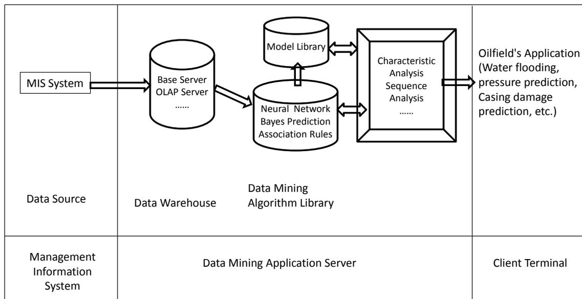
Figure 32 Data Mining Application System
