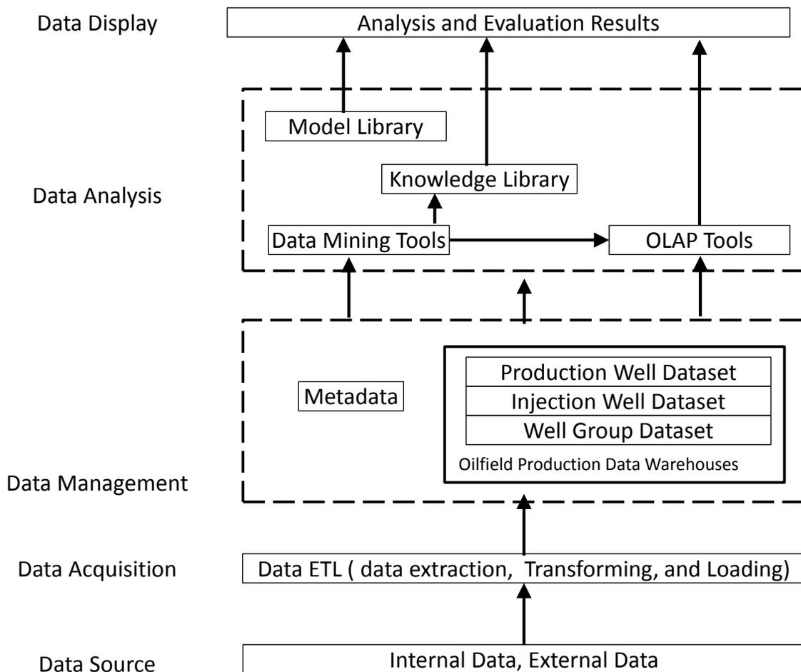
Figure 33 the Architecture of Data Warehouse of Oilfield Production Decision Support System
