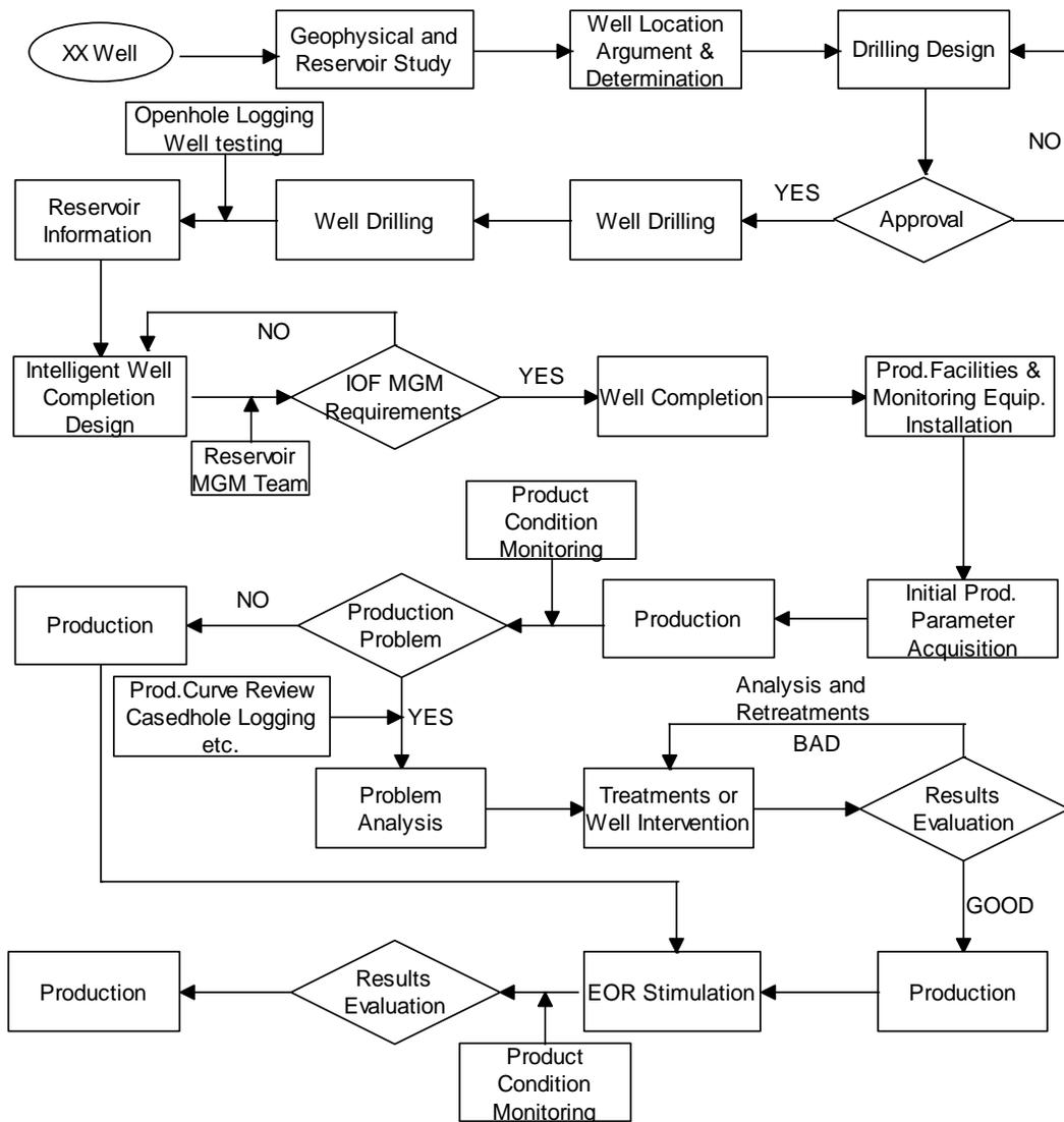
Figure 30 an Optimized Work Process of Well Production Management
