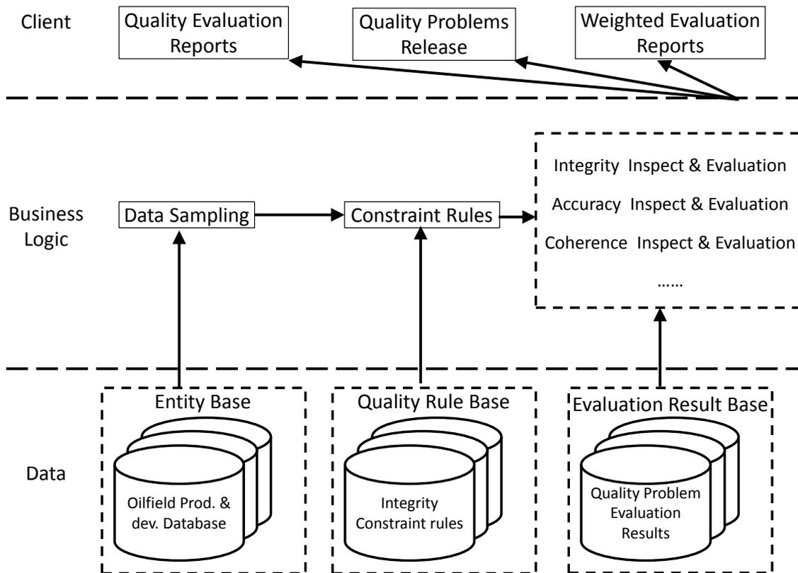
Figure 31 Rule-based Quality Inspection & Evaluation Model
