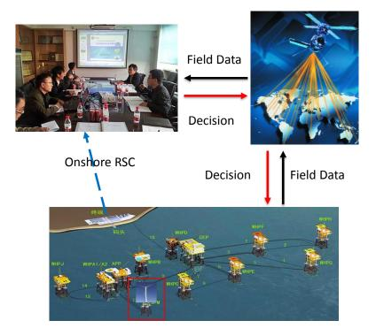
Figure 24 the Schematic of Data Transmission in CNOOC
