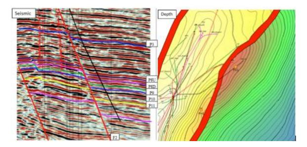
Figure 36 Seismic-Profile over Well PH-X and 2D Well Track Projection
