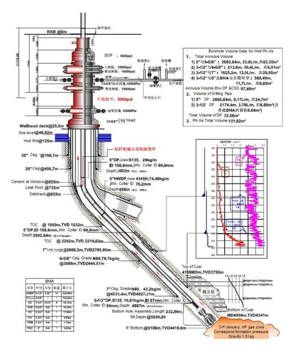
Figure 37 Well Schematic of Well PH-Xs
