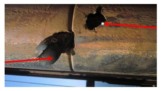
Figure 41 Photo of DP String Damage in Well PH-Xs
