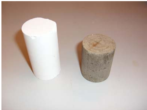
Figure 4.1. Chalk core and limestone core The chalk core used was outcrop chalk from Stevens Klint. Figure 4.1 shows a chalk core and a limestone core. The limestone core 20A was chosen because it had approximated the same permeability as the chalk core. All limestone cores had been used in previous experiments, thereby the permeability and porosity was known. The cores that had been used in previous experiments had all been washed by the same washing method. This washing method is described later in this chapter 4.1.4.
