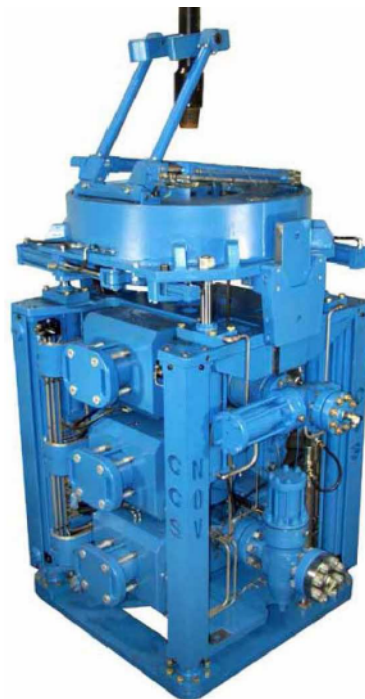
Figure 15 – The main unit of the Continuous Circulation System[23].
