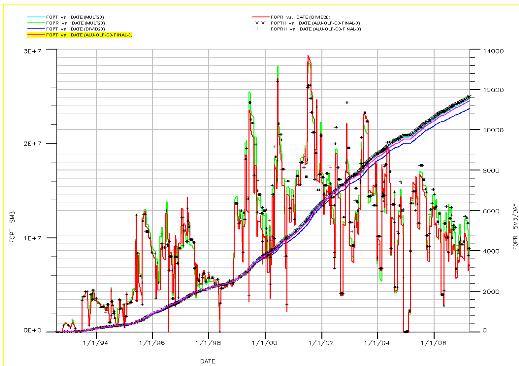
Figure 8-2 Total oil production match and oil production rates match for MULT20 and DIVD20
