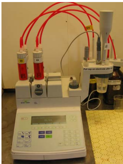
Figure A.7: Measurement of AN and BN by a titrator.
