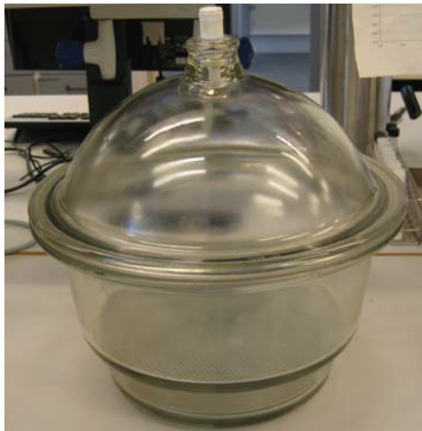
Figure 3.6: Lowering of initial water saturation by a desiccator.
