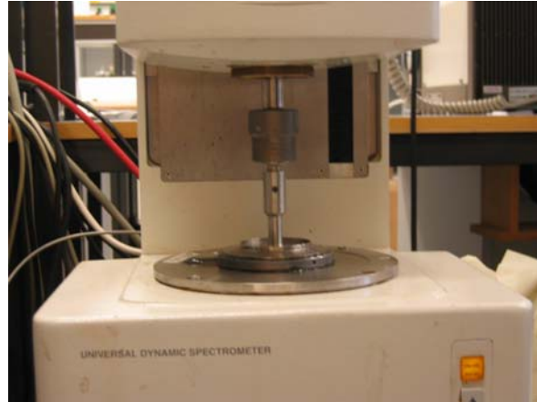
Figure 3.2: Measurement of viscosity by a spectrometer.
