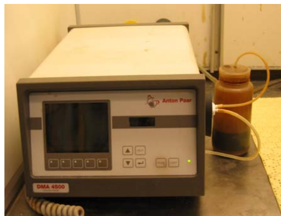
Figure 3.3: Measurement of density by a densitometer.
