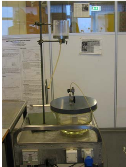
Figure 3.4: Saturation of core under vacuum.
