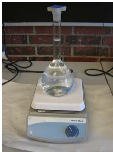
Figure A5: The brines were stirred with a magnetic bar.
