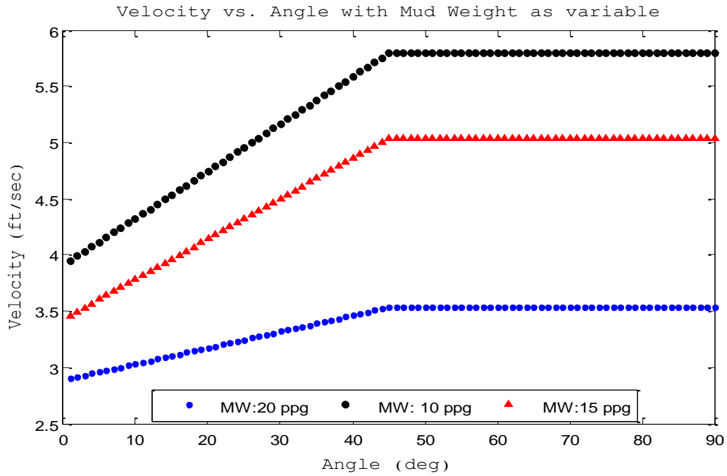
Figure (C.1): Minimum flow velocity vs. angle of inclination when the mud weight varies.
