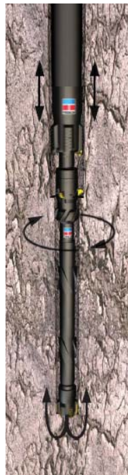
Figure 42 - Casing drilling has the ability to rotate and reciprocate while circulating fluid [56].
