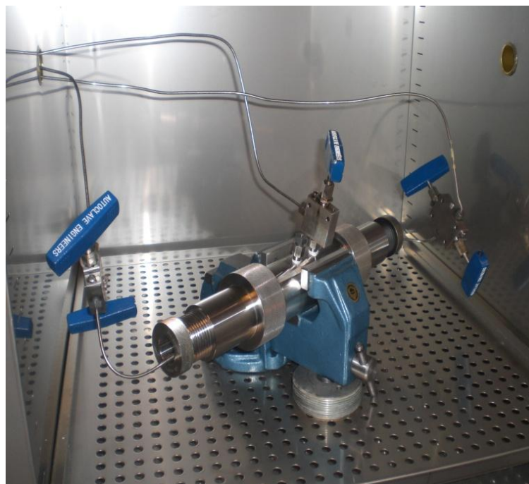
Figure 3.1 Picture of a Hassler cell.
