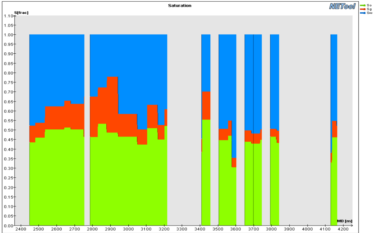
Saturation plot, showing the oil (green), gas (red) and water (blue) saturations
