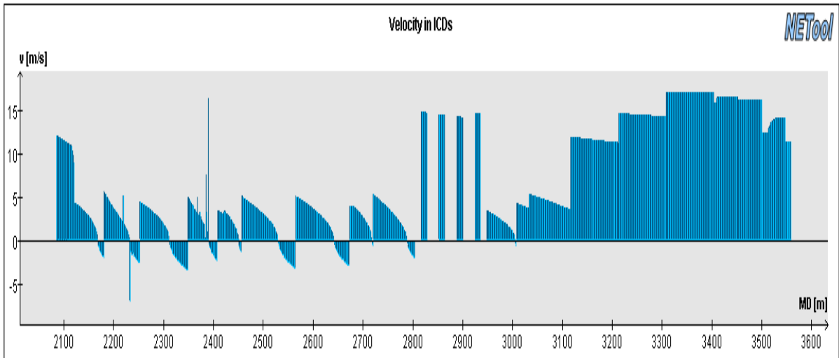
Velocity of the flow in the Annulus, tubing and through the ICDs
