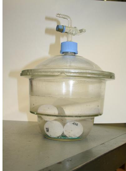
Figure 3.1: The desiccator that was used to saturate the core plugs.
