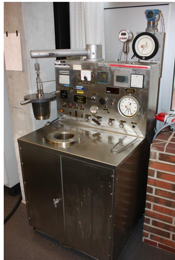
Figure 6: The pressurized consistometer used for testing thickening time at constant pressure (E.S. Keeling)
