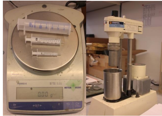
Figure 5: Left: Examples of syringes used. The weight used measures down to 0.01 grams. Right: A Chan 85 rotational viscometer used for rheology testing. (E.S. Keeling)
