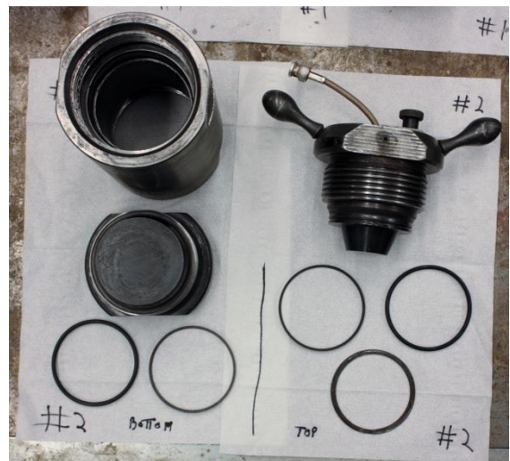
Figure 9: Details of the test cell that is installed in the UCA apparatus during testing. (E.S. Keeling)
