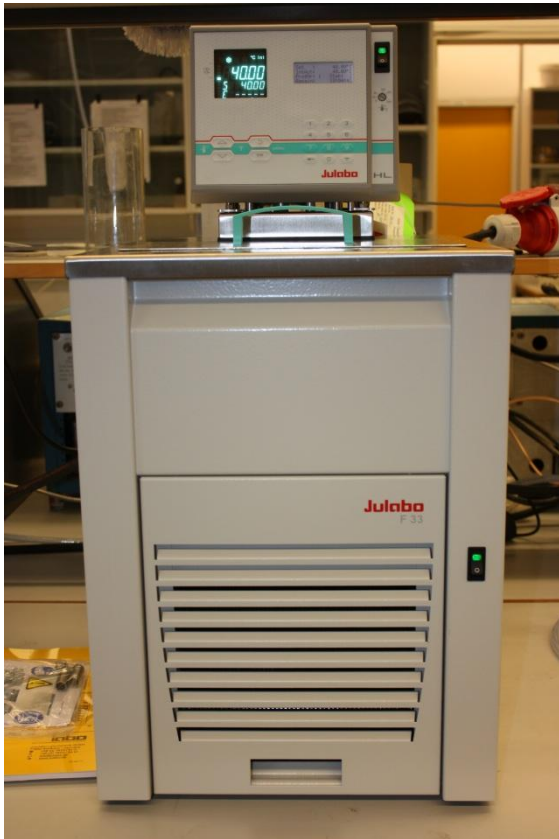
Figure 7: A programmable Julabo heat/cooling bath used for simulating temperature during thickening time tests and compressive strength tests. (E.S Keeling)
