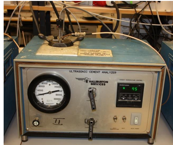
Figure 8: The Ultrasonic Cement Analyzer used for compressional strength tests. (E.S. Keeling)
