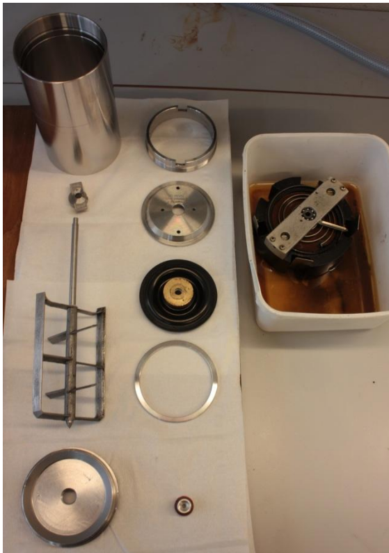
Figure 18: The components of the cell placed inside the pressurized consistometer. (E.S. Keeling)
