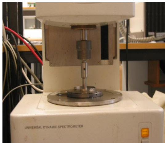
Figure A.4: Viscosity measurement on a Universal Dynamic Spectrometer
