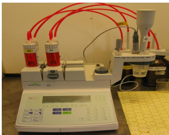
Figure A.5: Automatic titrator for measuring the AN and BN of the oil samples.
