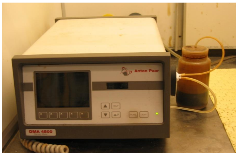
Figure A.3: Density measurement on a DMA 4500 Density Meter
