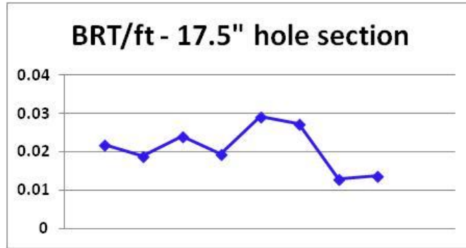
Graph 23 - The development of BRT hrs/ft chronological arranged in time for the 17 ½ "hole section.
