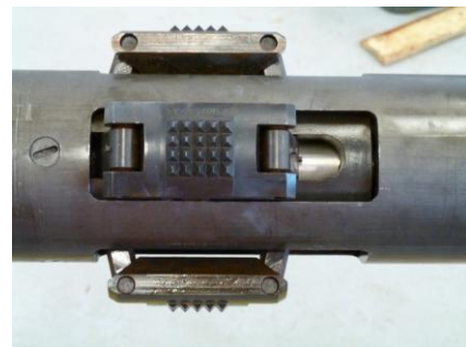
Figure 9.2 – Anchor and stoker module incorporated in the CannSeal tool. [67]
