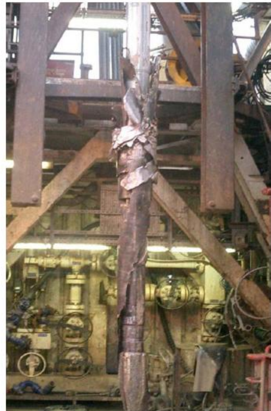
Figure 7.10 – “Skimmed casing” - Metal cuttings can cause failure of the milling assembly. [54] Copyright 2011, Society of Petroleum Engineers Inc. Reproduced with permission of SPE. Further reproduction prohibited without permission.
