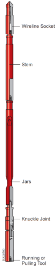
Figure 4.2 – Wireline toolstring. (Courtesy of Halliburton.) [22]
