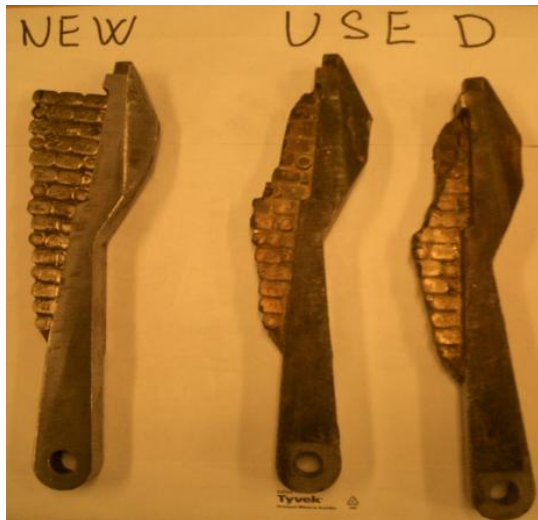
Figure 7.11 – New and worn out milling blades. [57]
