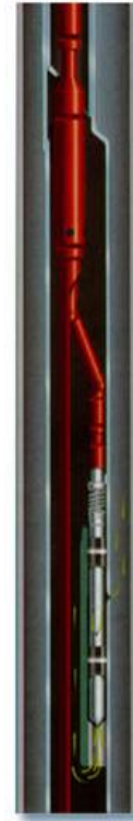
Figure 5.8 – Kickover tool retrieving GLV or dummy valve from a side pocket mandrel. (Courtesy of Weatherford.) [38]
