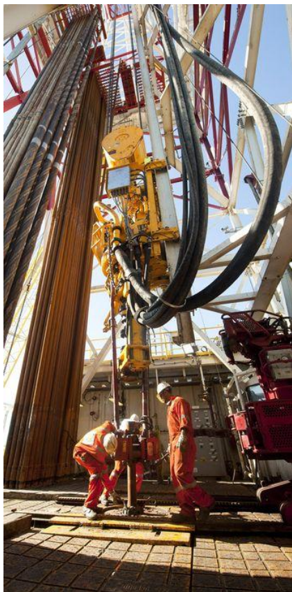
Figure 4.8 – A topdrive located within a derrick. The iron roughneck, mud injection hoses, pipe racks and the travelling blocks can also be seen. [34]
