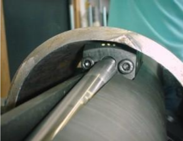
Figure 9.3 – Injection module incorporated in the CannSeal™ Tool. [67]
