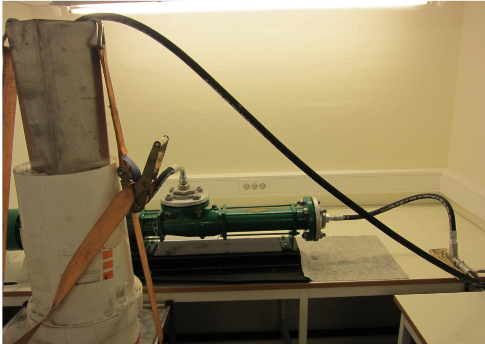
Figure 17: Final rig up of the laboratory foam generator loop.
