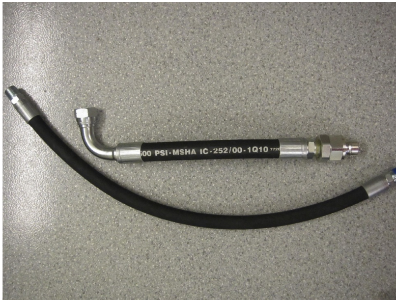
Figure 11: Foam Loop Hoses
