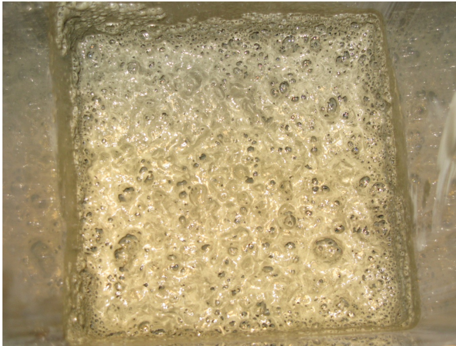
Figure 18: Bubbles at surface right after foaming, test 1.
