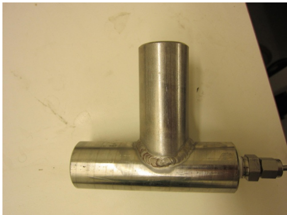
Figure 16: Foam Tee Generator with nitrogen supply connected.
