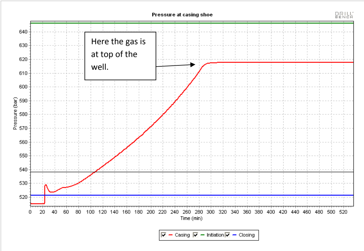
Figure 67: Casing shoe pressure, closed in well with WBM.
