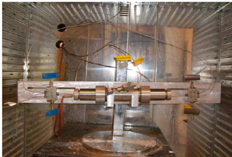
Figure 4.1 Core cleaning setup
