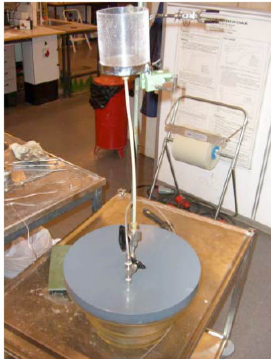
Figure 4.2 Evacuating and saturating the core with formation brine[2]
