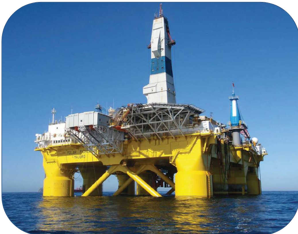
Fig. 48 Transocean Polar Pioneer semi-submersible drilling rig (Source: Transocean)
