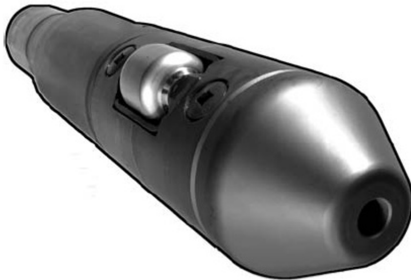
Figure 2-23 Rotary compliant expansion tool (Innes et al., 2004)
