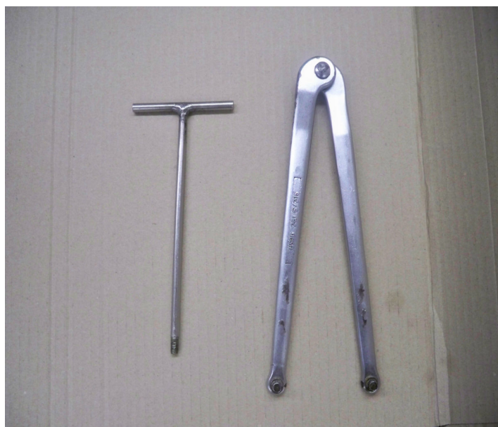
Fig. 3.11 Tools for removing end seal and end cap
