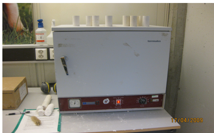
Fig.3.2 The heating cabinet
