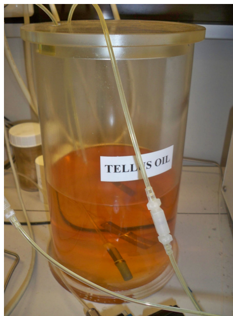
Fig. 3.12 Hydraulic oil used by the Gilson pump.
