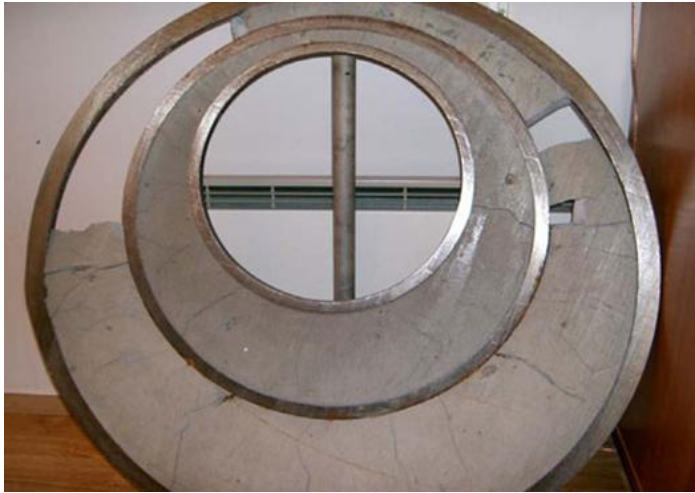
Figure 25: Bad casing centralization (WellCem, 2012)
