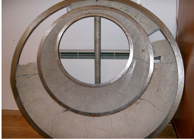
Figure 3.8.1.2: Cement that is fractured between casing strings after the steel has been heated up and then cooled down. [Wellcem, 2009]
