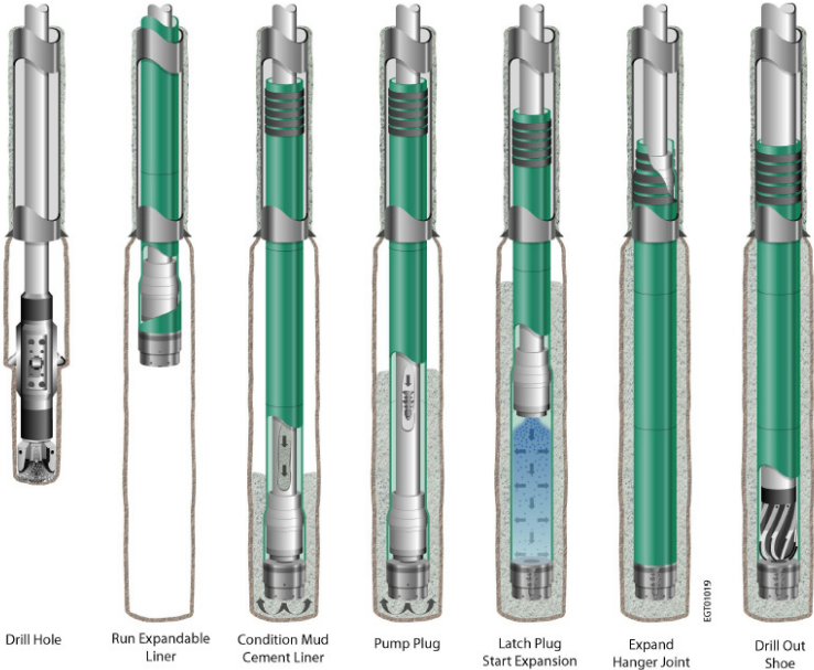
Figure 3.3.2.2: Principle of expandable liner. [DeMong and Rivenbark, 2003]
