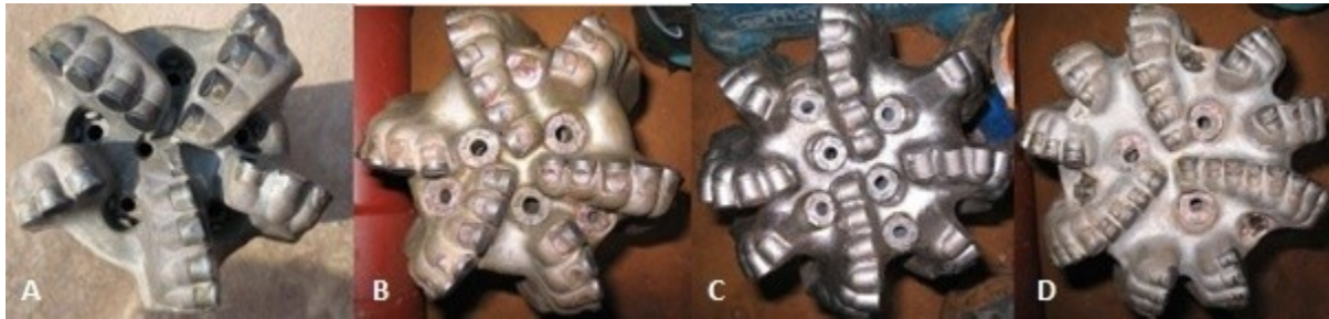
Figure 3.7 The design of PDC bits depending on the hardness of the rocks (from soft A to hard D) 7 .
