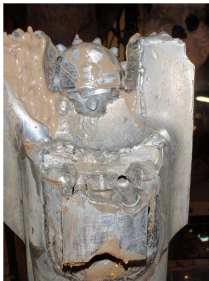
Figure 4.3 Worn out bit from section 8 ½” 17 .
