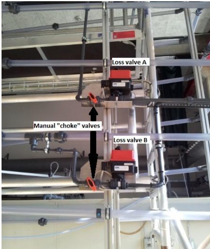
Automatic loss valves in closed position. Manual “choke” valves adjusted to allow desired efflux cross section.
