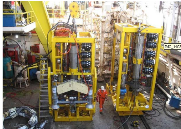
Figure 32: Upper and lower subsea pumps 13
