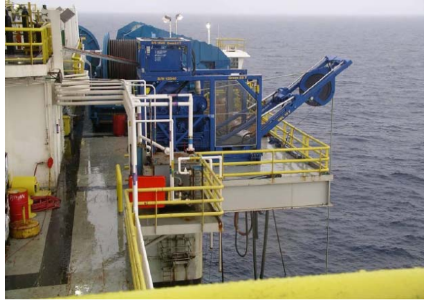
Figure 34: Winch for umbilical 13
