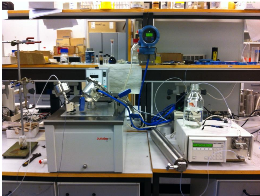
Figure 3.1: The setup for measuring the shrinkage factor of oil at 110° C and 23°C.
