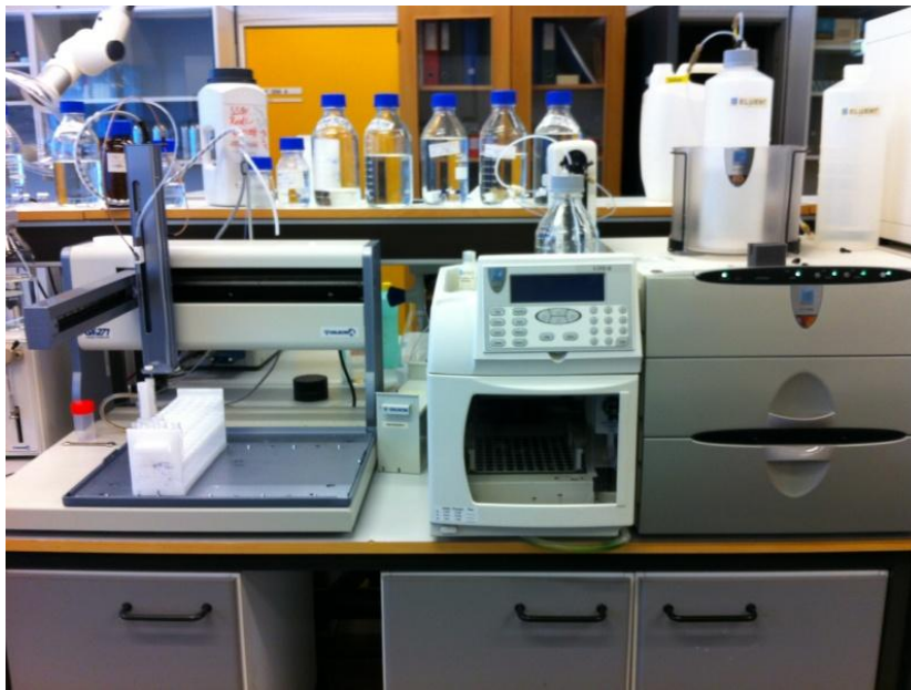
Figure 3.7: To the left; machine to perform dilutions of sample tests. To the right; IC (Ion Chromatograph) for performing chemical analysis of sample tests.
