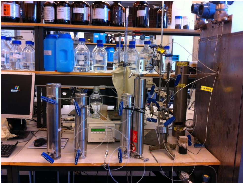
Figure 3.6: Setup for flooding. The piston cells seen from the left contained Yme FW, SW, d_{50} SW and oil saturated with \text{CO}_2 .
