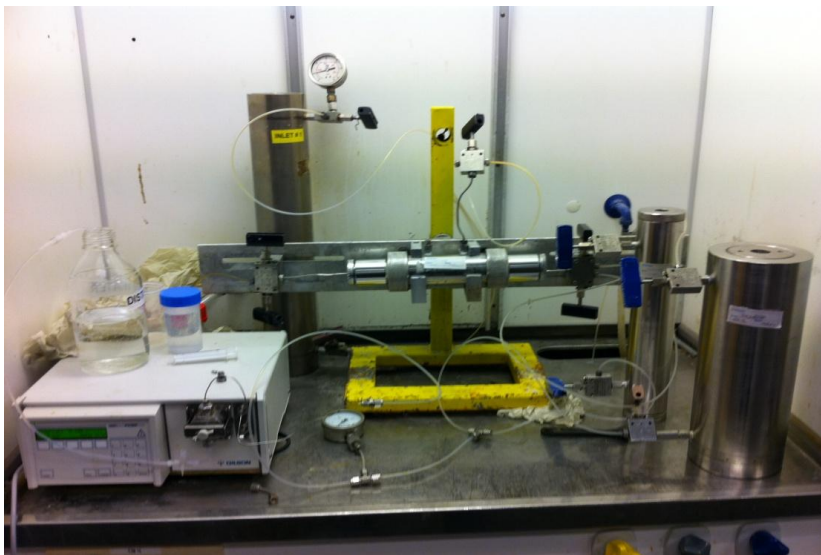
Figure 3.2: Core cleaning setup.
