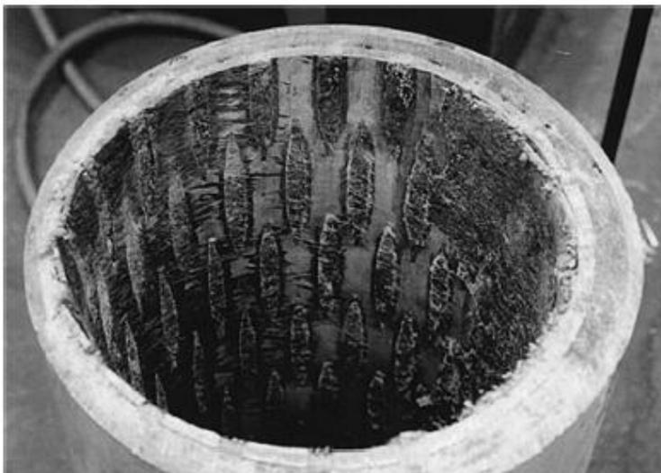
FIGURE 6: DRILLED OUT SECTION OF EST IN FIBER CEMENT (STEWART , GILL ET AL. 1996)
