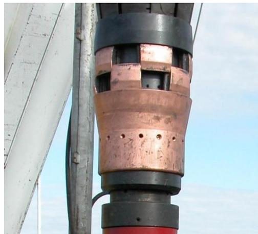
FIGURE 18: TWO STAGE EXPANSION CONE (BAKER HUGES, 2011)
