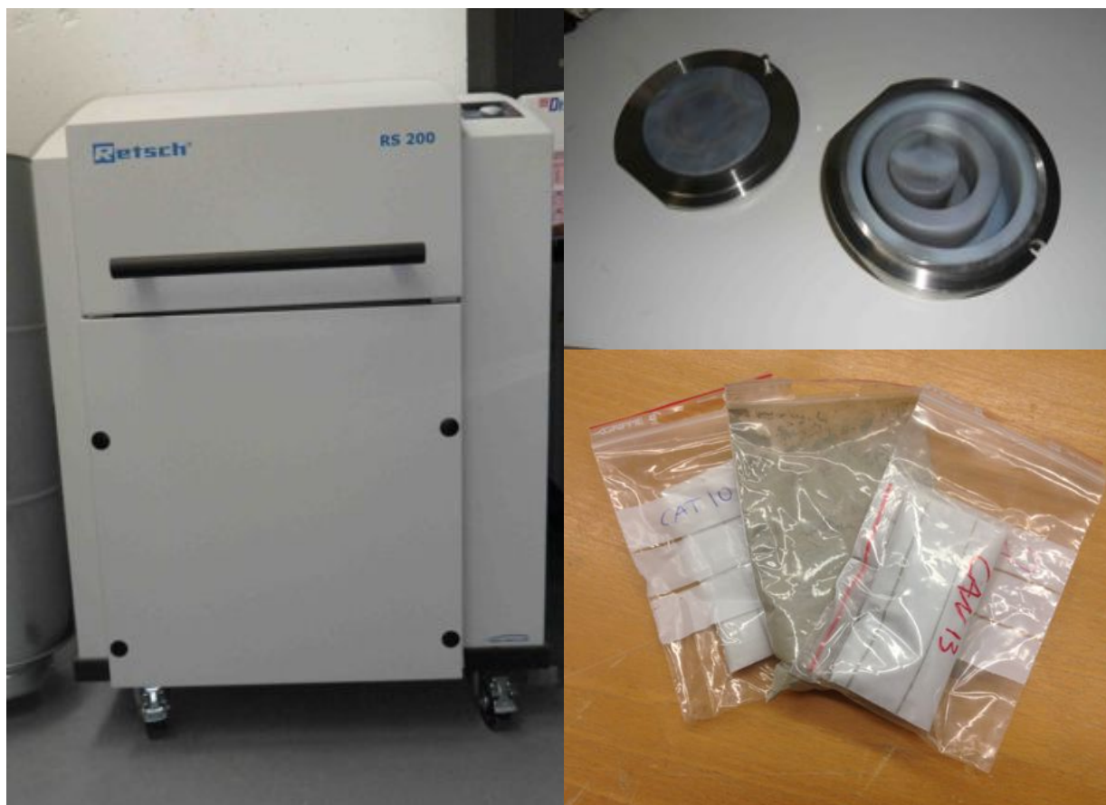
Fig. C 1 – Milling process. Right: Retsch RS200 automated milling machine, Upper right: Beakers used during the milling process. Lower left: Milled material bagged and tagged, ready for geochemical and TOC measurements.
