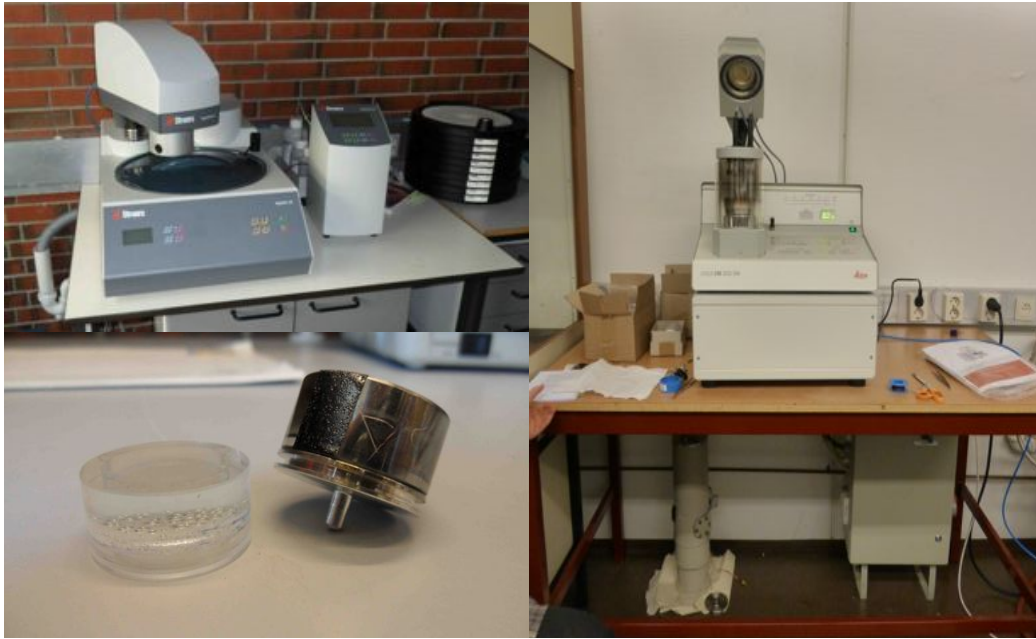
Fig. C 3 – Upper left: Struers TegraPol-35 automated polishing machine. Right: Leica EM SCD500 high vacuum sputter coater. Lower left: Polished heavy mound containing heavy mineral fractions and coated mound fixed to aluminum peg with carbon tape ready for SEM analysis.
