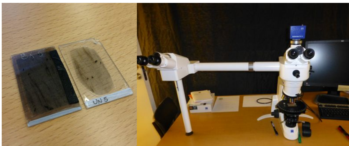
Fig. C 2 – Left: Thin sections, prepared for analysis. Right: Zeiss AXIO light microscope with an AxiCam ERc 5s camera connected to a computer.
