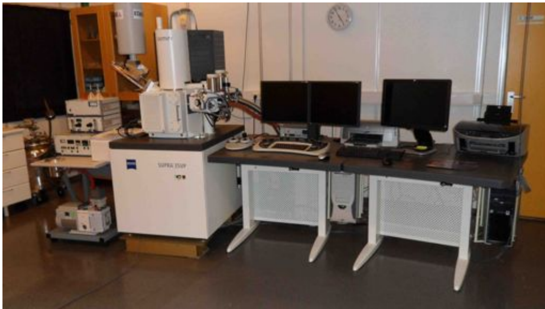
Fig. C 4 - Left: Zeiss Supra 35 VP featuring a Scanning electron microscope (SEM) with a Back scattered electron (BSE) detector, Cathodluminescence (CL) and a Energy dispersive spectrometer (EDS). To the right, three screens used for visualizing the fractions and analysing EDS results.
