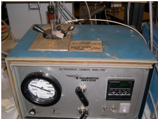
Figure 4: UCA and steel test cell with temperature control, pressure supply and signal transducer connected.
