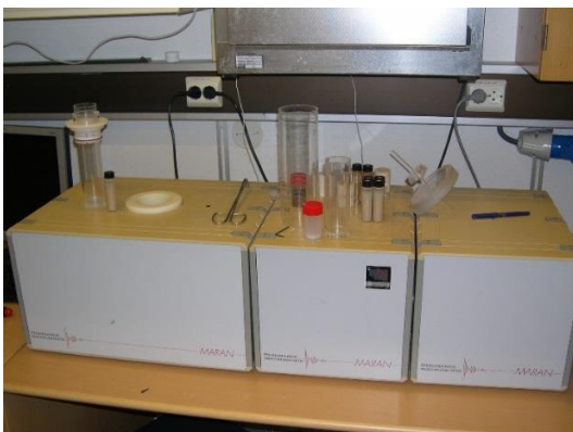
Figure 5: NMR instrument and test tube filled with Halliburton OBM.
