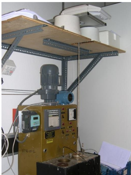
Figure 3: Direct weight measurement setup consisting of a modified atmospheric consistometer connected to a laboratory scale by a steel rod.
