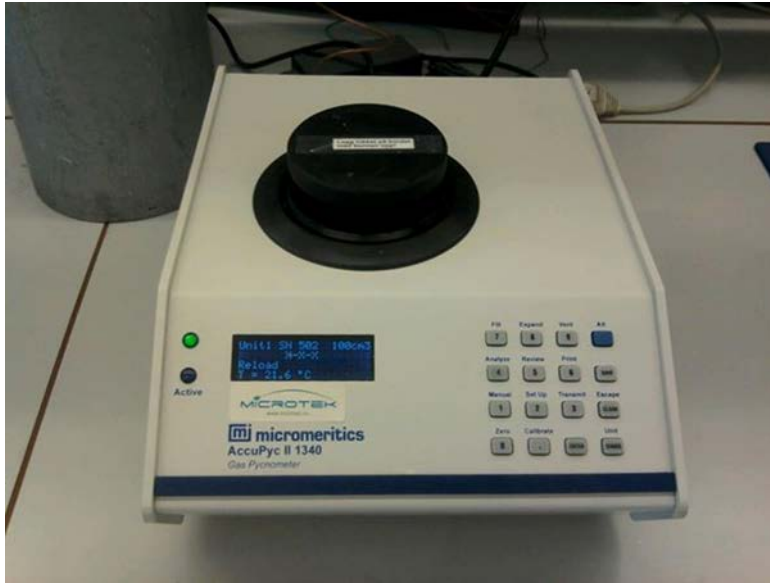
Figure 3.4: Gas Pycnometer was used to measure the volume of the cores. Based on the volume measured and the weight of the cores, the densities of the cores were calculated.
