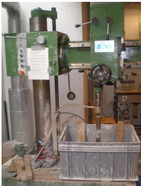
Figure 3.1: The drilling machine used to extract the cores from the Mons chalk block.
