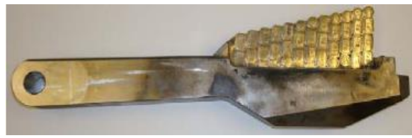
b. Section Blade with 'P' cutters
