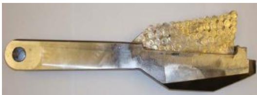
a. Section Blade with traditional cutters
