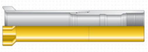
Figure 31: Liner Setting Sleeve [37]
