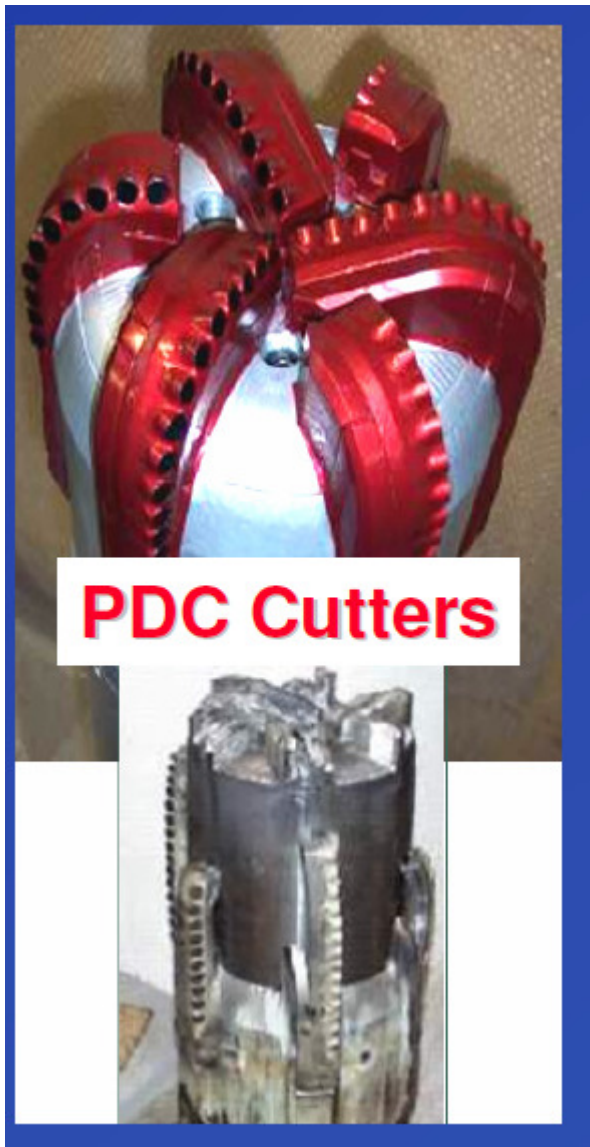
Figure 16: PDC Casing Drilling Bit Pre- and Post-Expansion [26]
