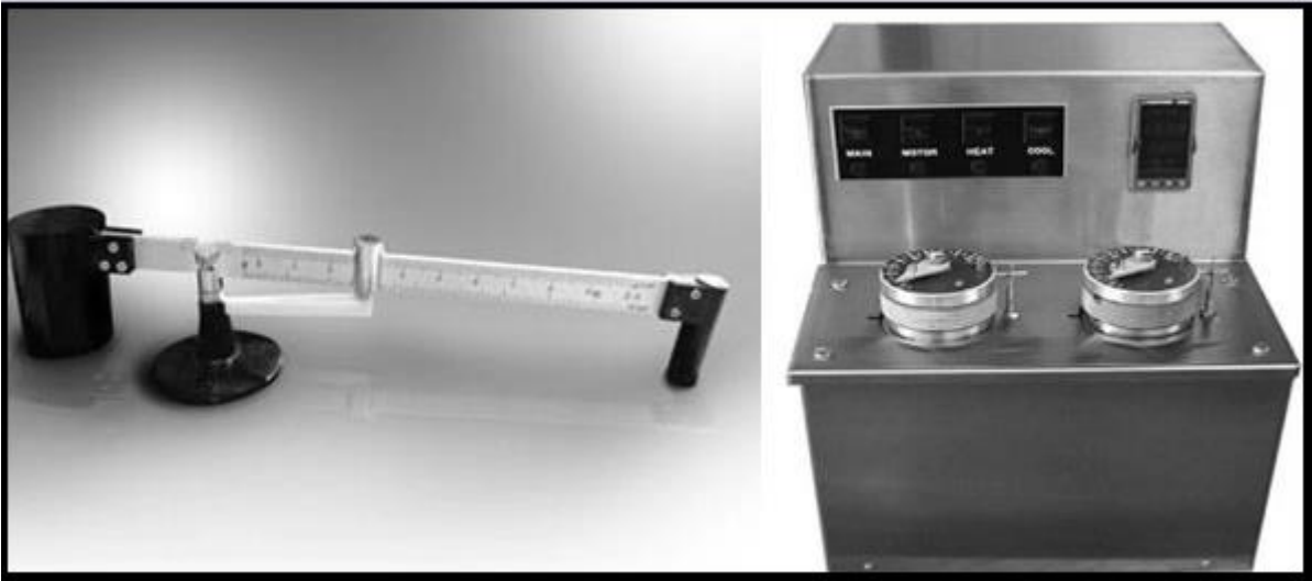
Picture 7.4 a common fluid density balance on the left and an atmospheric conditioning meter to the right in the picture [32] [34].
